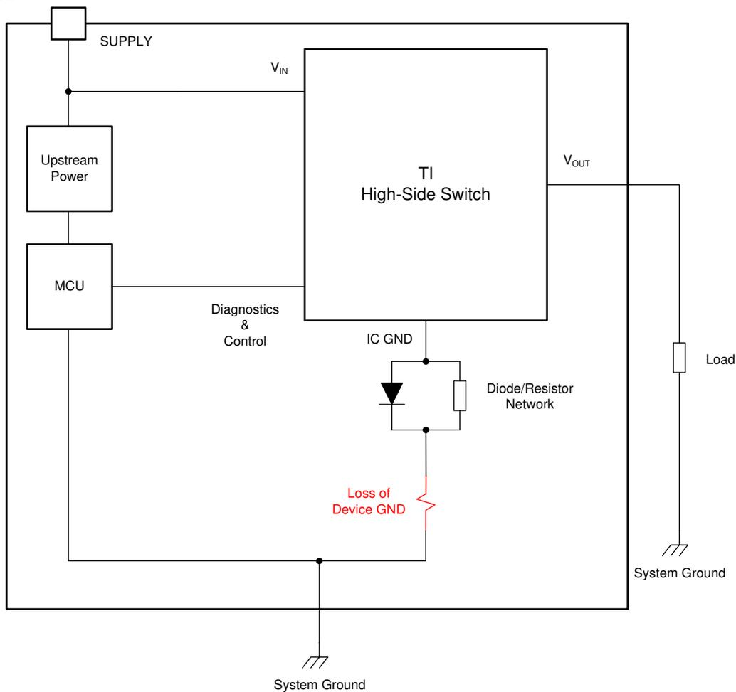
**Figure 1-1. Loss of Device Ground**
