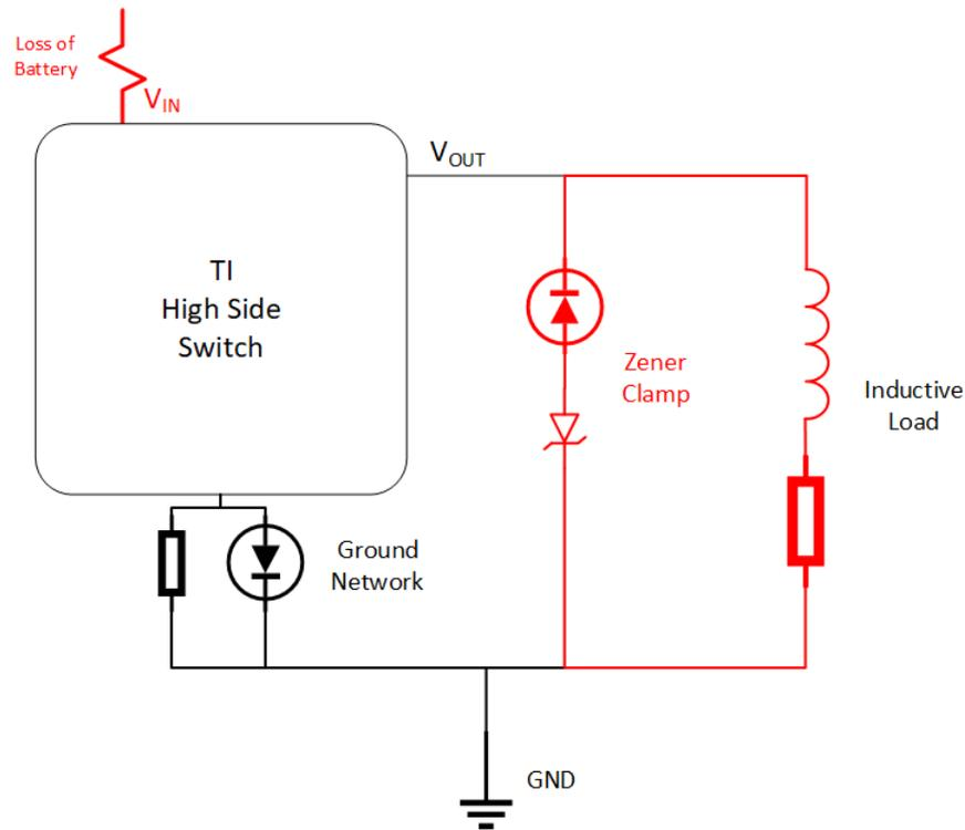
**Figure 2-2. Zener Diode for Inductive Loading**
