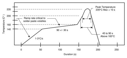
Figure 1-1. Starting Profile for Typical Pb/Sn Solder Paste
