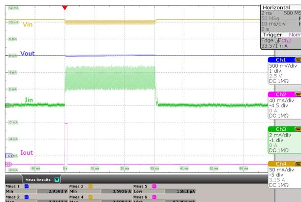
**Figure 6. 2.5-mA ICL With 100-mA Load Step**
