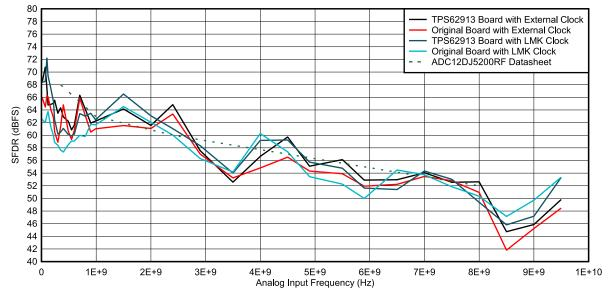
Figure 2-7. Spurious-Free Dynamic Range Comparison Graph
