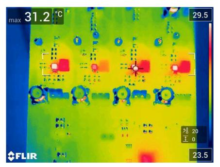
Figure 2-13. TPS62913 Switching Converters
