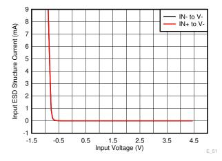
Figure A-11. OPA310 - Setup 3 - ESD Diode Current for Applied Input Voltage
