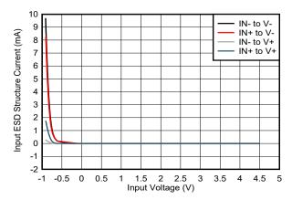
Figure A-9. TLV341/TLV341A - Setup 2 - ESD Diode Current for Applied Input Voltage
