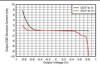
Figure A-10. TLV341/TLV341A - Setup 2 - ESD Diode Current for Applied Output Voltage
