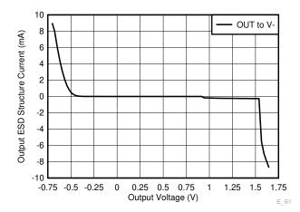
Figure A-12. OPA310 - Setup 3 - ESD Diode Current for Applied Output Voltage
