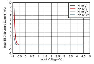
Figure A-19. TLV341/TLV341A - Setup 4 - ESD Diode Current for Applied Input Voltage
