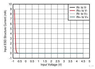
Figure A-1. OPA310 - Setup 1 - ESD Diode Current for Applied Input Voltage
