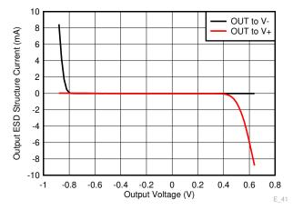
Figure A-8. OPA310 - Setup 2 - ESD Diode Current for Applied Output Voltage
