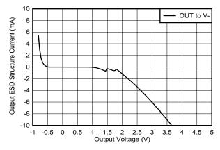
Figure A-14. OPA348 - Setup 3 - ESD Diode Current for Applied Output Voltage
