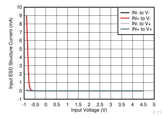
Figure A-17. OPA310 - Setup 4 - ESD Diode Current for Applied Input Voltage
