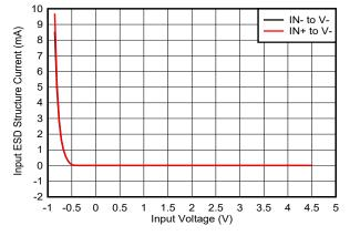
Figure A-13. OPA348 - Setup 3 - ESD Diode Current for Applied Input Voltage
