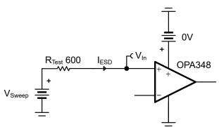
Figure 3-2. OPA348 - Test Setup of ESD Structure Current for Extended Applied Input Voltage
