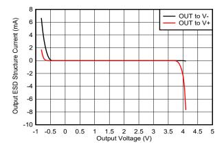
Figure A-20. TLV341/TLV341A - Setup 4 - ESD Diode Current for Applied Output Voltage
