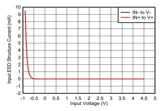
Figure A-15. TLV342/TL342A - Setup 3 - ESD Diode Current for Applied Input Voltage
