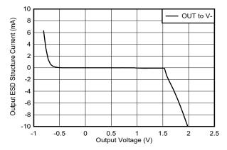
Figure A-16. TLV342/TLV342A - Setup 3 - ESD Diode Current for Applied Output Voltage
