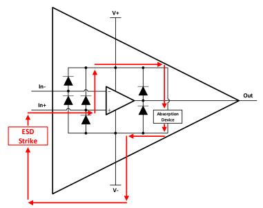
Figure 2-1. Path of Current During ESD Strike From In+ to V– for Op Amp With Standard ESD Protection
