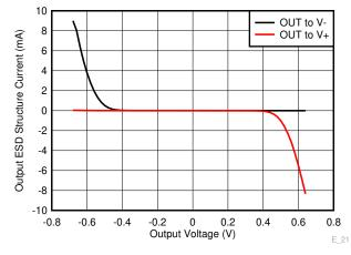
Figure A-2. OPA310 - Setup 1 - ESD Diode Current for Applied Output Voltage
