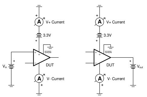
Figure 4-4. Setup 4 - Example Schematic for Testing IN+ and OUT Pins With Power on V+ Pin, Grounded V- Pin and Shutdown Pin Low
