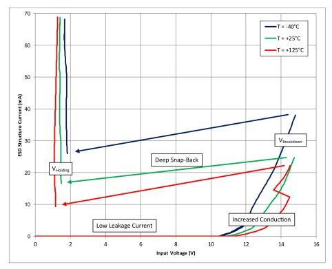
Figure 3-3. OPA348 - ESD Structure Current for Extended Applied Input Voltage
