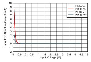
Figure A-5. TLV342/TLV342A - Setup 1- ESD Diode Current for Applied Input Voltage
