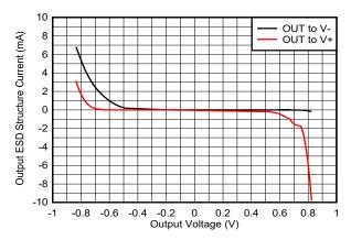
Figure A-6. TLV342/TLV342A - Setup 1 - ESD Diode Current for Applied Output Voltage
