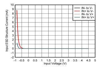
Figure A-3. OPA348 - Setup 1 - ESD Diode Current for Applied Input Voltage
