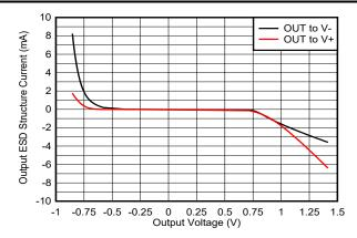
Figure A-4. OPA348 - Setup 1- ESD Diode Current for Applied Output Voltage
