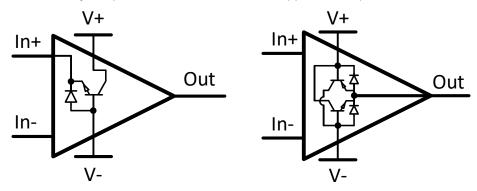
Figure 3-1. Current Paths for IN+ (also present for IN-) and OUT
