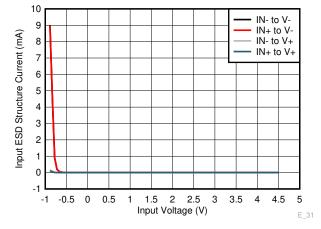
Figure A-7. OPA310 - Setup 2 - ESD Diode Current for Applied Input Voltage
