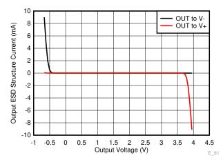
Figure A-18. OPA310 - Setup 4 - ESD Diode Current for Applied Output Voltage
