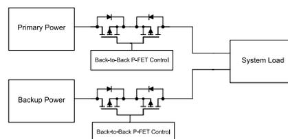
Figure 2. Discrete P-Channel MOSFET Power MUXing Configuration
