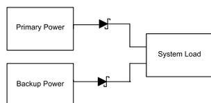
Figure 1. Diode ORing Configuration
