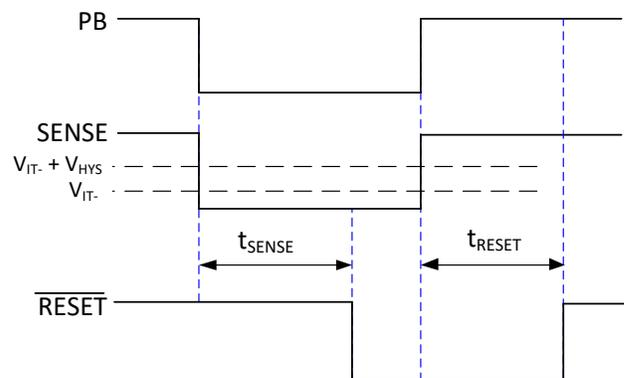
**Figure 2. Programmable Push-button Circuit Timing Diagram**
