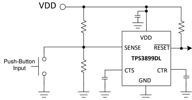
**Figure 1. Programmable Push-button Circuit Using TPS3899**
