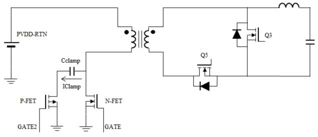
Figure 1-1. Active Clamp Forward Design
