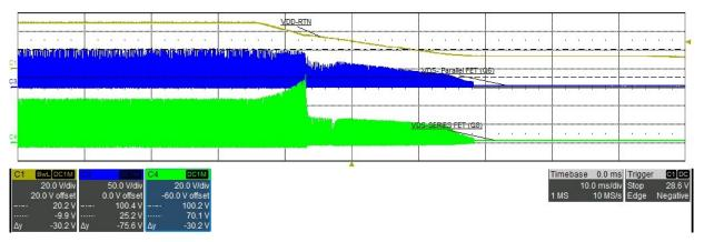
Figure 3-10. Soft-Stop Enabled No Load Secondary MOSFETs
