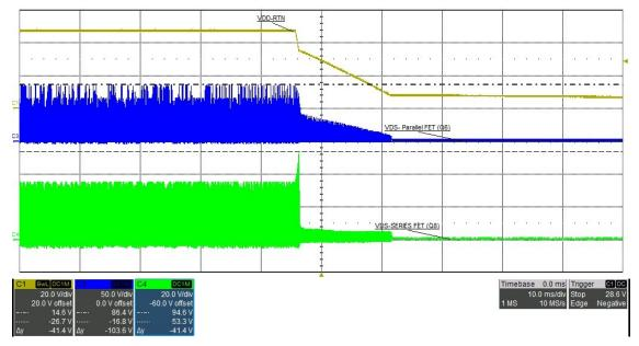
Figure 3-6. Soft-Stop Enabled Full Load for Secondary MOSFETS
