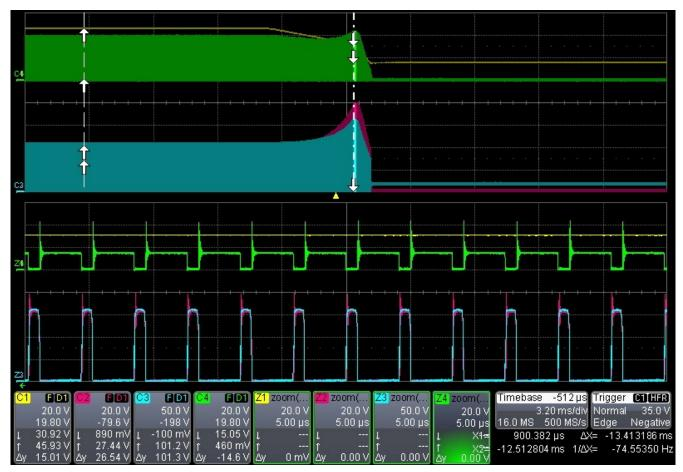
Figure 2-1. Active Clamp Forward Shutdown Sequence Without Soft-Stop
