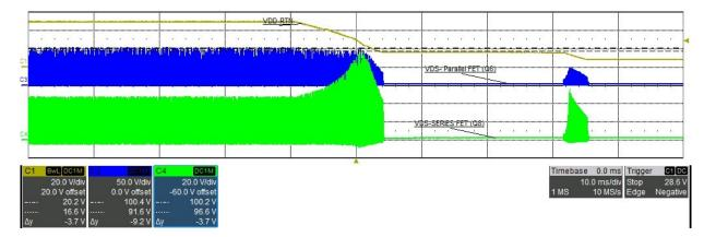
Figure 3-11. Soft-Stop Enabled vs. Disabled Full Load for Secondary MOSFETs
