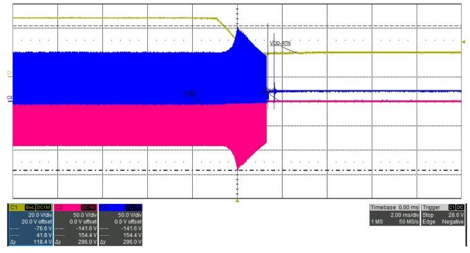
Figure 3-5. Soft-Stop Disabled Full Load for Primary MOSFETs
