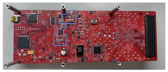
Figure 1-4. Image of bottom of Original board with Switchers and LDO's outlined in Blue
