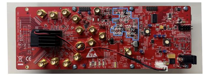
Figure 1-6. Image of top of Revised board with TPS541620 and TPS62913 Switchers outlined in Blue
