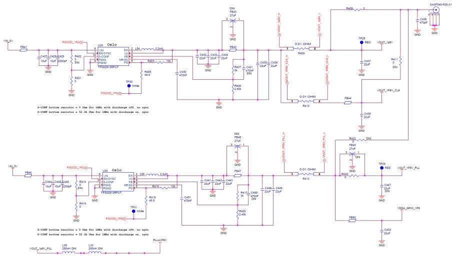
Figure 3-1. TPS62913 1.8 V Power Schematic
