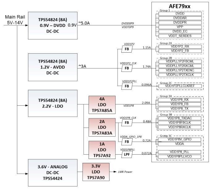
Figure 1-2. Original Power Block Diagram for AFE7920 RevC Evaluation Module
