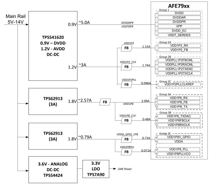
Figure 1-5. Power Block Diagram for AFE7920 Rev C Evaluation Module with TPS62913
