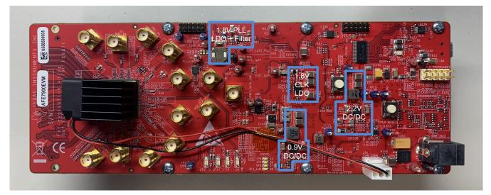
Figure 1-3. Image of top of Original board with Switchers and LDO's outlined in Blue
