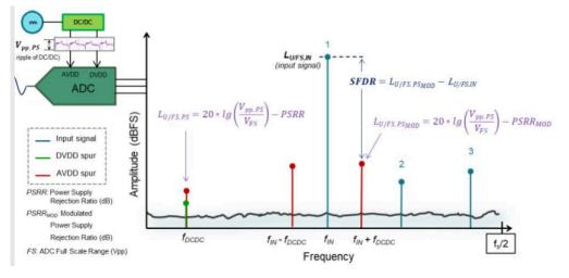
Figure 1-1. Power supply noise and ripple in the ADC output spectrum
