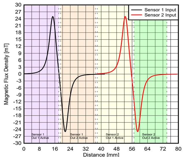
**Figure 5. Two-Sensor Input**
