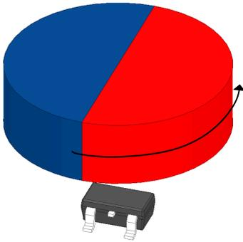
**Figure 7. TMAG5110 On-Axis**
