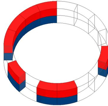
**Figure 9. Coded Magnetic Wheel**
