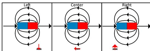
**Figure 4. Magnetic Field for Three-Position Switch**
