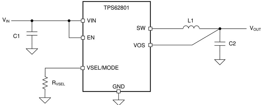
Figure 4-1. TPS62801 Typical Application Schematics
