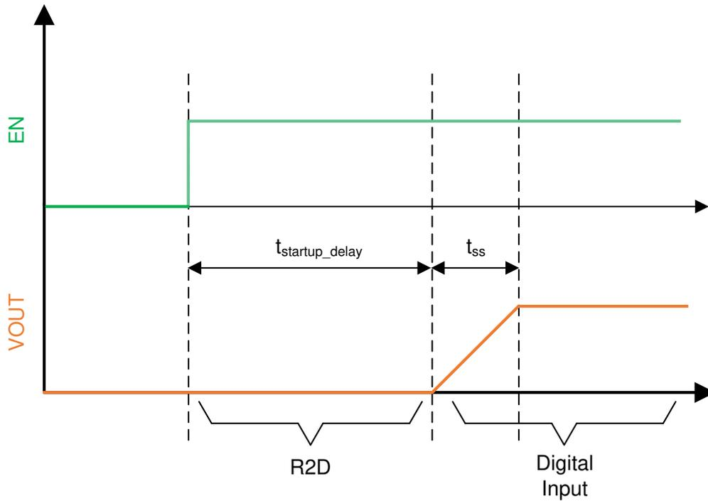
**Figure 1-2. VSET/MODE Pin Time Multiplexing**
