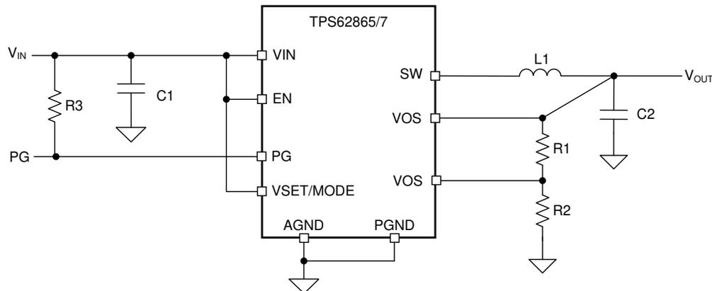
**Figure 5-2. Typical Application Schematics TPS62865/7 – Forced PWM operation**
