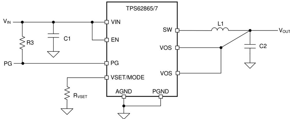
**Figure 5-1. Typical Application Schematics TPS62865/7 – Fixed Output Voltage**
