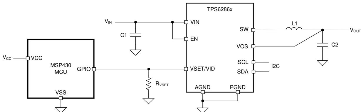
Figure 3-1. Typical Application Schematics, VSET/VID Driving Circuit with MCU
