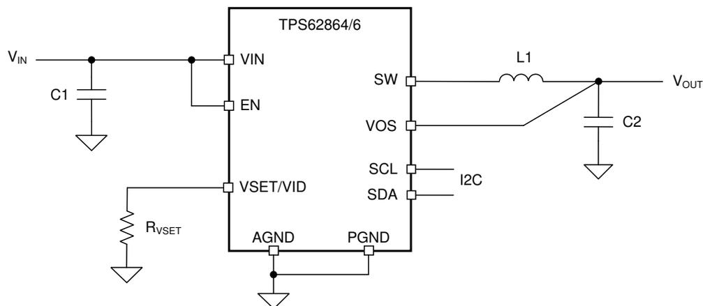
**Figure 1-1. TPS62864/6 Typical Application Schematics**
