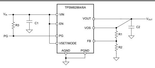
Figure 5-4. Typical Application Schematics TPSM82864/6A - Forced PWM Operation
