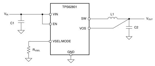
Figure 4-1. TPS62801 Typical Application Schematics
