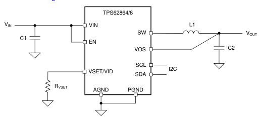
Figure 1-1. TPS62864/6 Typical Application Schematics
