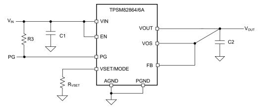
Figure 5-2. Typical Application Schematic TPSM82864/6A - Fixed Output Voltage
