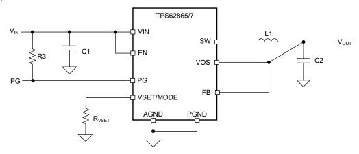
Figure 5-1. Typical Application Schematics TPS62865/7 - Fixed Output Voltage
