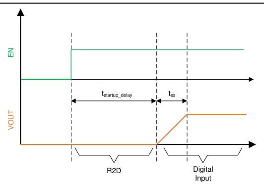
Figure 1-2. VSET/MODE Pin Time Multiplexing
