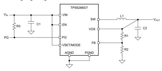
Figure 5-3. Typical Application Schematics TPS62865/7 - Forced PWM Operation
