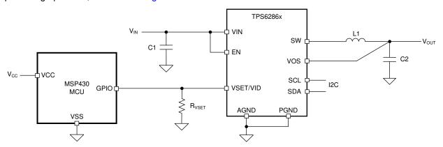
Figure 3-1. Typical Application Schematics, VSET/VID Driving Circuit with MCU
