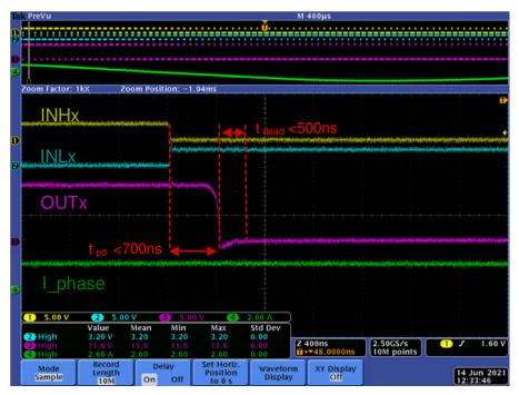
Figure 2-6. Waveforms of Dead Time and Propagation Delay When INHx is Falling, INLx is Rising, and Current Flows Out of OUTx
