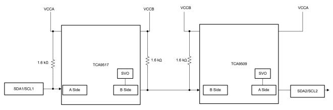
Figure 2-3. Schematic of Proper Implementation of Buffers With SVO
