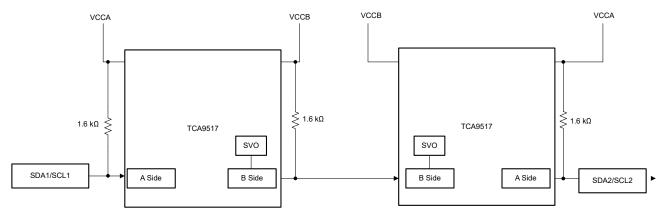
Figure 2-1. Schematic of Improper Implementation of Two TCA9517s
