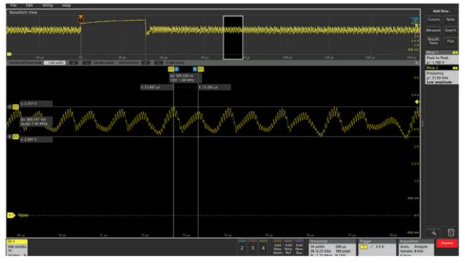
Figure 3-2. Bench Test With 1nF C\_sink
