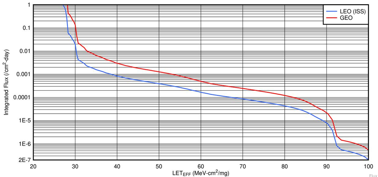
Note that the y-axis represents flux integrated from higher LET to lower LET. The value of integral flux at any specific LET value is actually the integral of all ion events at that specific LET value to all higher LETs.
