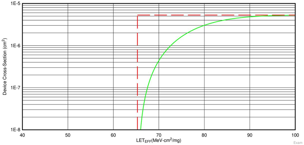
**Figure 1-2. Device Cross Section Versus LET<sub>EFF</sub> Showing How the Weibull Fit (Green) is “Simplified” With the Use a Square Approximation (Red Dashed Line)**
