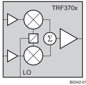
Figure 1. TRF370x Functional Block Diagram
