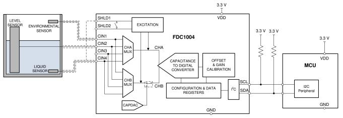
Figure 2-2. FDC1004 for Liquid Level Measurements
