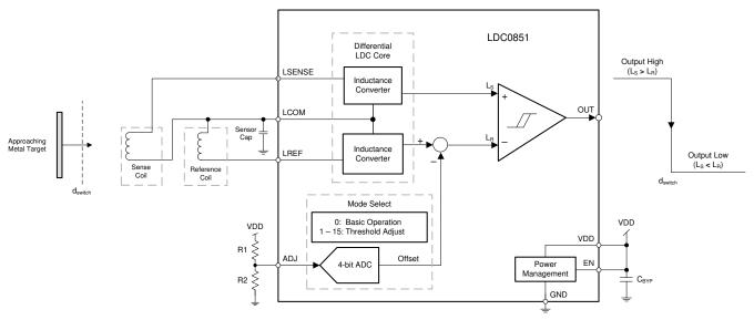
Figure 4-3. LDC0851 Functional Block Diagram
