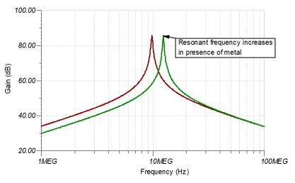
Figure 1-2. Resonant Frequency Shift in Presence of Metal
