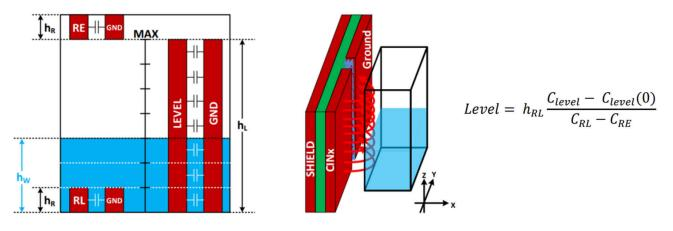
Figure 2-1. FDC Capacitive Level Sensing Application
