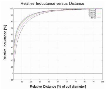
Figure 5-4. Relative Inductance vs Distance
