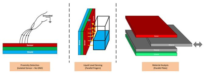
Figure 1-3. Capacitive Sensing Applications
