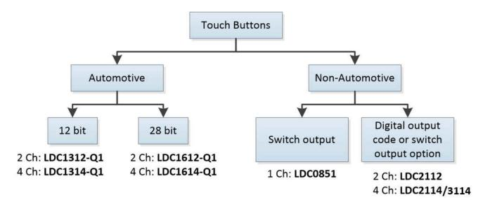
Figure 3-2. Inductive Touch Device Selection Flow Chart
