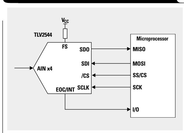
the sampling process has been completed. EOC returns to a high state upon the completion of the conversion process. When programmed as /INT, it can act as an interrupt to the host processor. /INT goes from a high to low state at the end of the conversion process and is cleared automatically on the following /CS falling edge.
