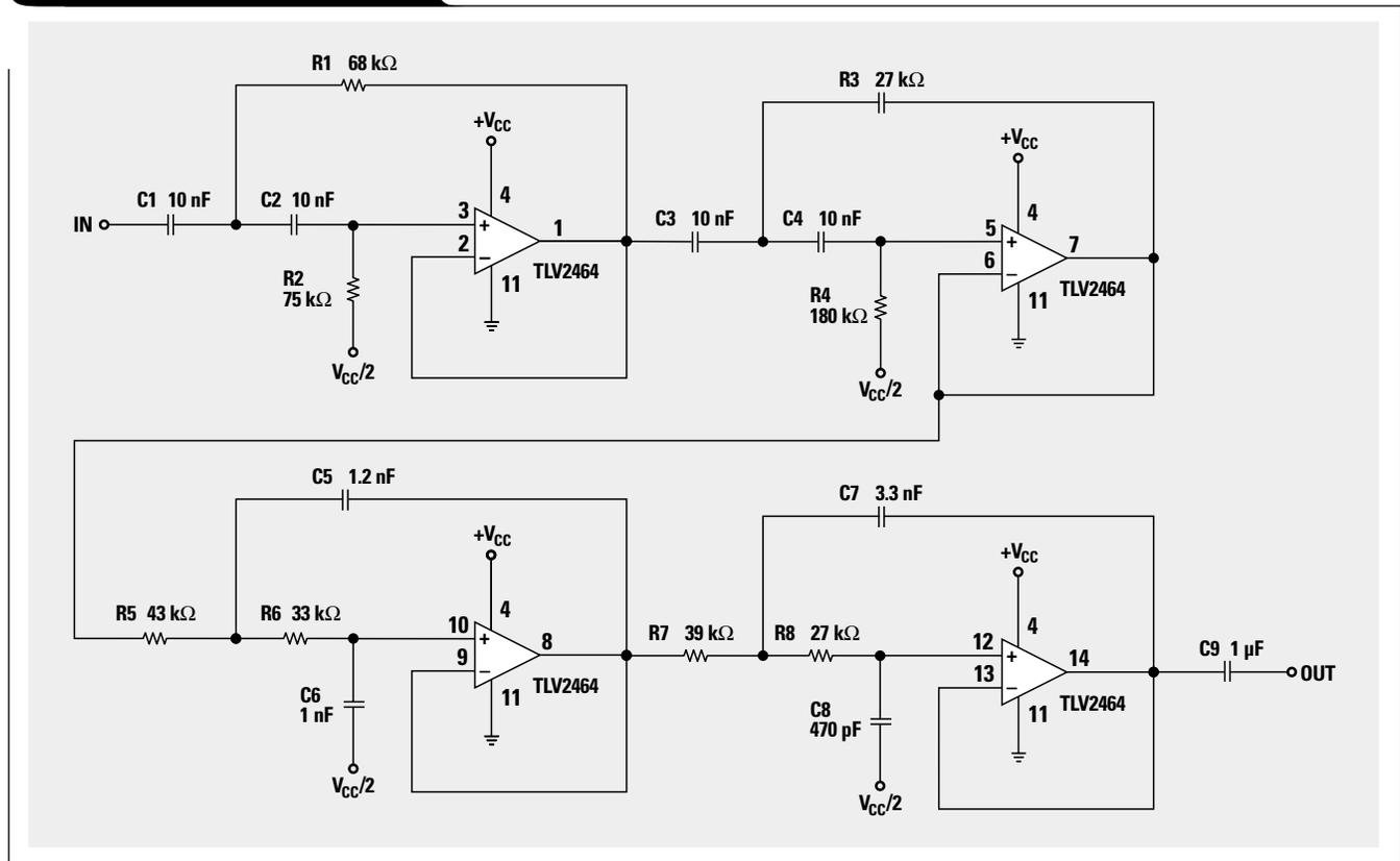
Figure 3 shows a second-order circuit. Nearby out-of-band signals, such as 60-Hz hum, are not rejected very well. This may be acceptable in cellular telephone headsets, but may not be for large switchboard consoles. A fourth-order speech filter, although more complex, can be implemented in a single quad op amp (with an external VCC/2 reference).
