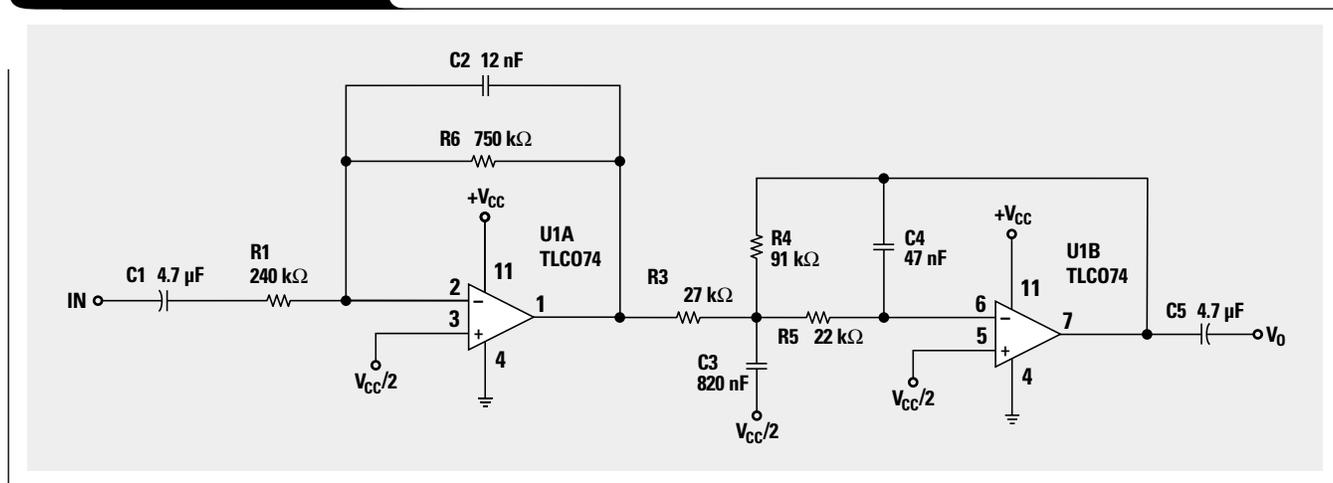
There is no stereo separation of low bass frequencies, and either channel (or both) can be used to drive the subwoofer circuit (sum into an inverting input with a second C1 and R1).
