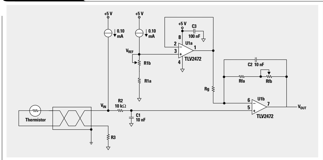
One of the two current regulators supplies  $100\ \mu\text{A} \pm 0.5\%$  to the thermistor. From resistance and current information, the thermistor voltage is  $0.06783\ \text{V}$  for  $100^\circ\text{C}$  and  $3.265\ \text{V}$  for  $0^\circ\text{C}$ .
