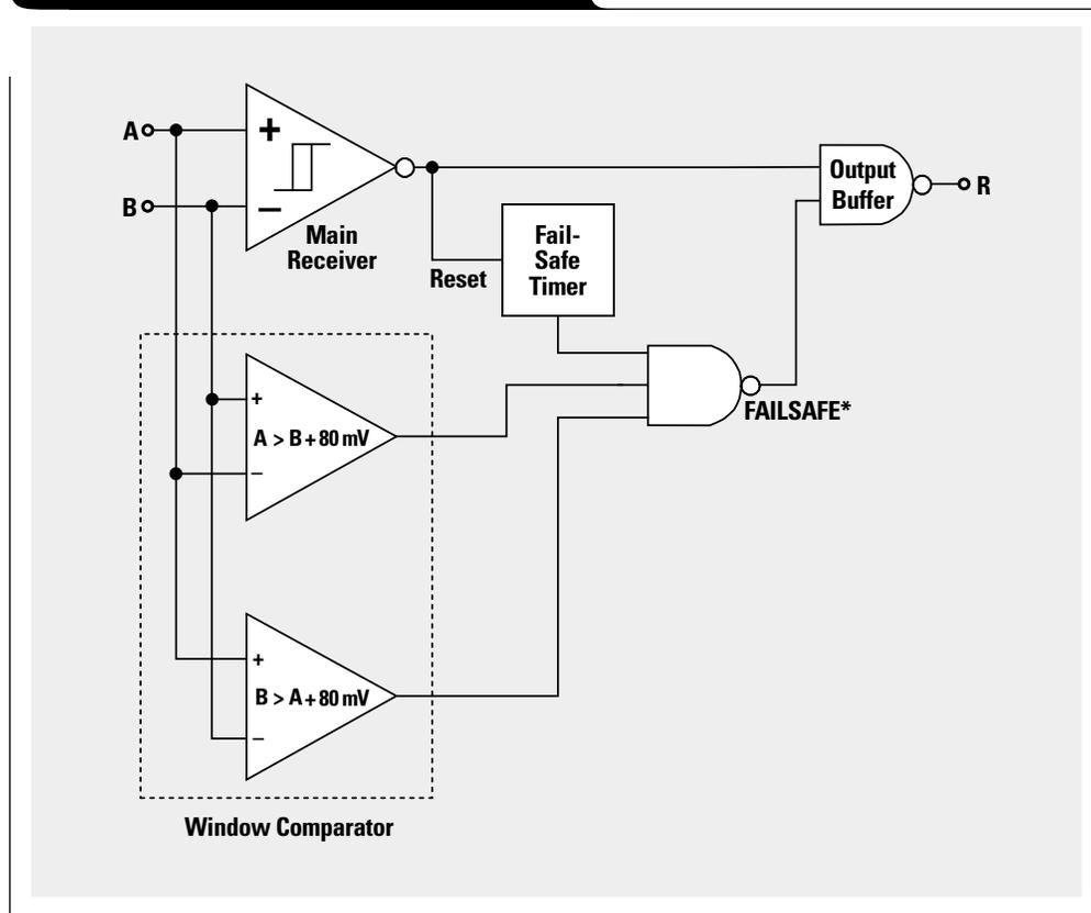
fail-safe threshold), FAILSAFE\* is not asserted, and output node R remains at logic LOW, tracking the input signal.
