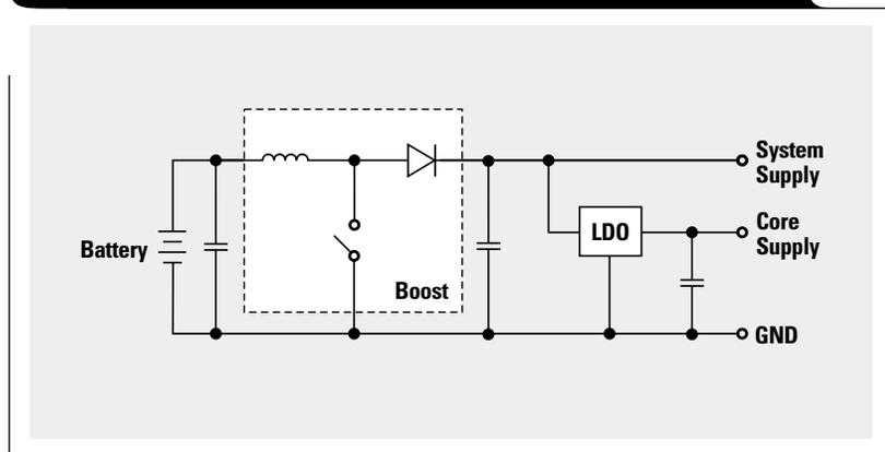
The standard boost converter shown in Figure 2 operates with one active switch, which is controlled by a pulse-width modulation (PWM) scheme. When the switch is closed, the inductor is charged by the battery. Opening the switch redirects the current through the rectifier to the output capacitor, which then is charged. The ratio between input and output voltages is determined by the duty cycle. Details about the design and operation of a boost converter can be found in References 1 and 2.
