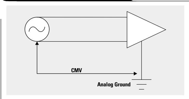
effects can be intermittent reboots, lockups, and bad data transfer. Network interface cards, serial ports, parallel ports, and modems are prime targets for some form of failure due to high CMV. If the CMV is high enough, component failure is possible.
