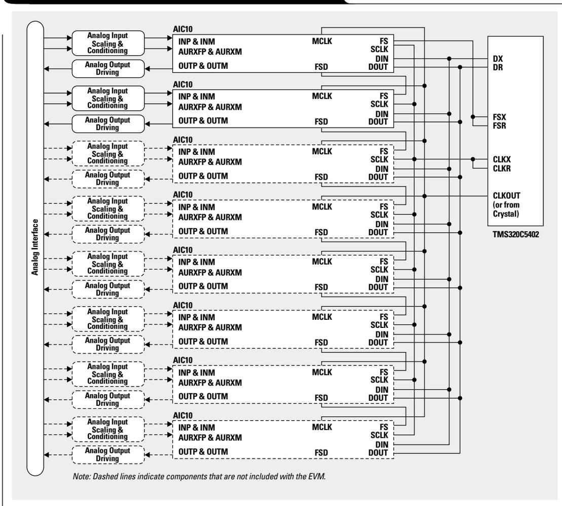
The TLV320AIC10 is a high-resolution, high-speed device that contains both ADC/DAC data paths. The ADC data path includes signal conditioning op amps, a multiplexer, an anti-aliasing filter, a programmable gain amplifier, a Sigma-Delta ADC, and a decimation filter. The DAC data path is composed of a glueless DSP interface to an interpolation filter, a Sigma-Delta DAC, a low-pass reconstruction filter, a programmable gain amplifier, and a transmit amplifier.
