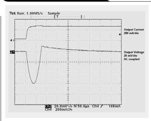
Figure 4. TPS75433 response to a 2-A-load transient
