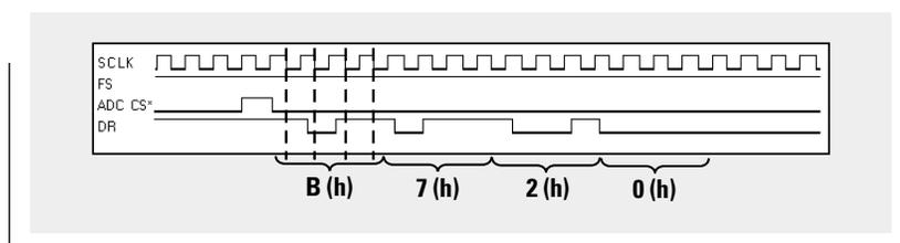
Figure 3. Conversion trigger timing in DSP mode
