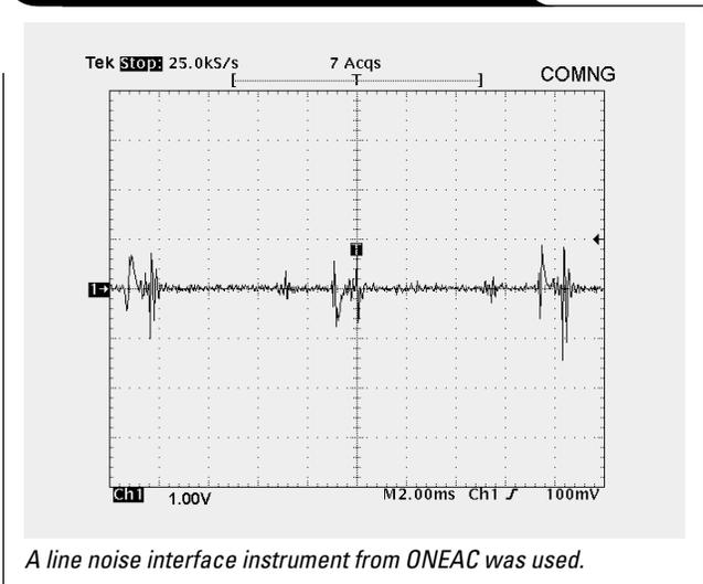
**Figure 2. Common-mode voltage**
