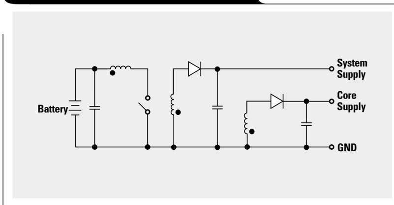
choosing the output that is regulated by the PWM controller that controls the flyback switch. When selecting the capacitors it is important to know that the input and output currents are discontinuous. Details about design and operation of flyback converters can be found in References 1 and 3.
