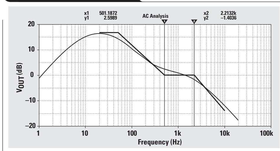
RIAA equalization curves often include another breakpoint at 10 Hz to limit low-frequency “rumble” effects that could resonate with the turntable’s tone arm. The standard input impedance in the circuits shown in Figure 10 is 47 k $\Omega$ . This impedance makes a convenient place to inject dc offset into single-supply circuits, so it is isolated from the phonograph cartridge by an input capacitance. The phonograph cartridge output is assumed to be 12 mV.
