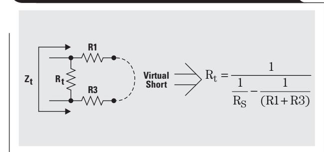
Once  $R_t$  is found, the required gain is found by generating a Thevenin equivalent circuit. The circuit is broken between  $R_t$  and the amplifier input resistors  $R_1$  and  $R_3$ .  $V_{IC}$  does not concern us at this point, so we will leave it out. Then
