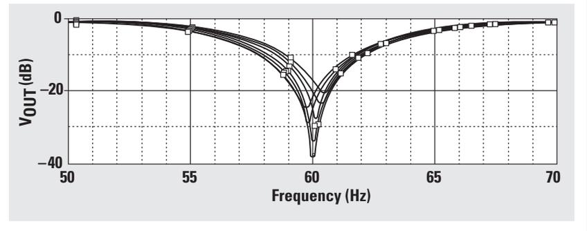
Figure 4. Response of a 50-Hz notch filter
