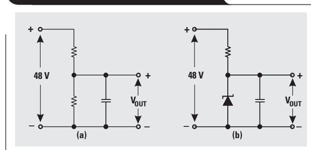
Of course, the performance of many other methods can equal or even surpass that of the Zener diode divider, but such methods tend to be more complicated and more expensive, and may be unnecessary for the –48-V applications. This is why the Zener diode divider is typically used in many 48-V hot-swap applications.
