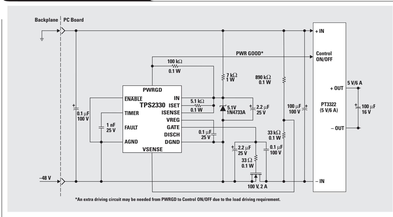
from TI. The main switch is a 100-V N-channel MOSFET, such as IRF530N.
