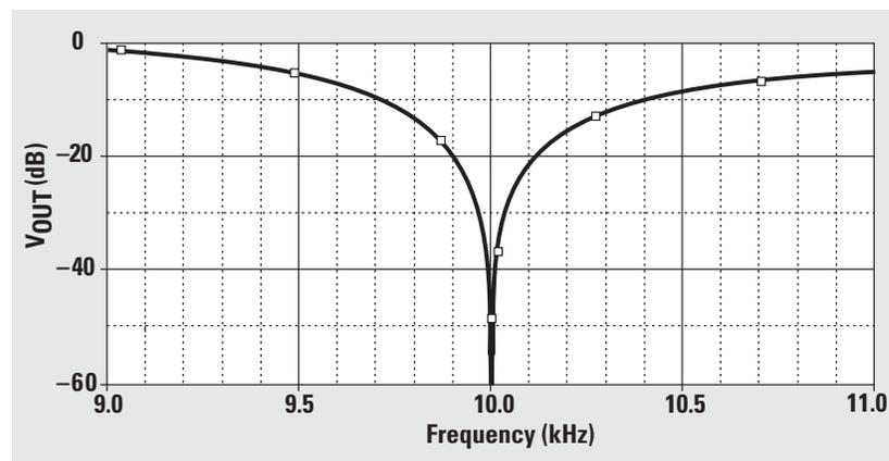
**Figure 7. Response of 9-kHz notch filter**
