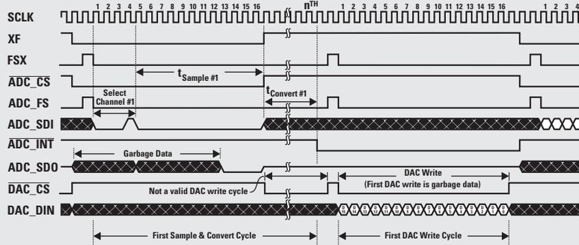
**Figure 10. ADC channel select, second generation cycle, and DAC write**
