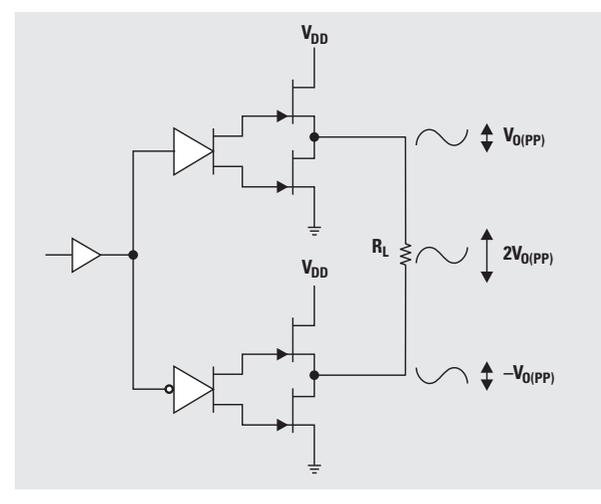
Figure 2. TPA6101A2 configured as a differential-input BTL Driver
