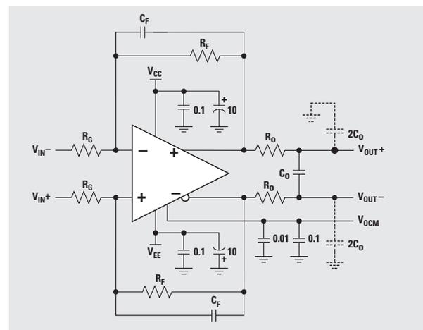
Figure 11. Third-order low-pass filter driving an ADC
