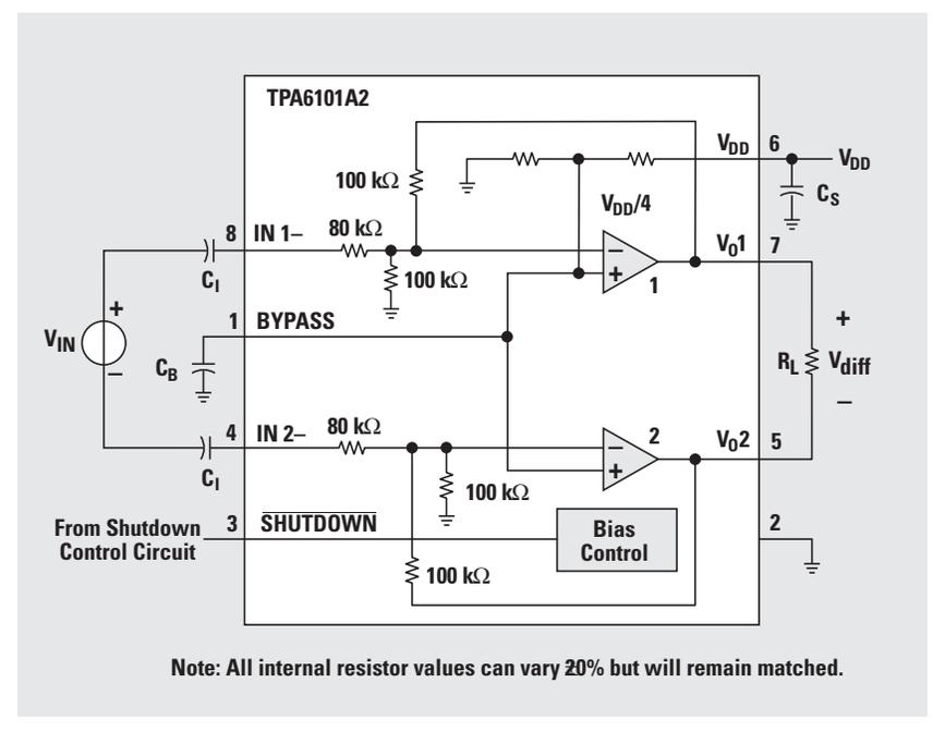
direction while the other output is moving in the negative direction. This effectively produces a voltage swing across the BTL that is two times the voltage swing seen across a
