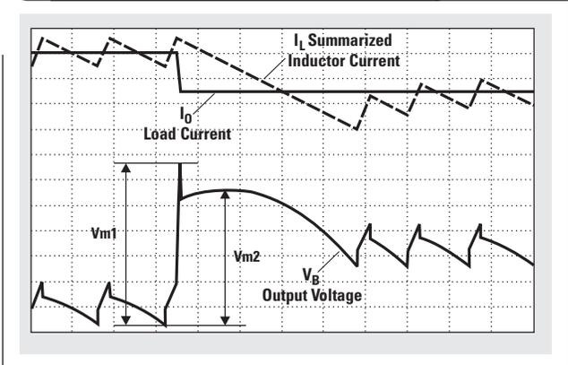
that the summarized inductor current and lower output voltage ripple need to be considered as they relate (in this analysis) to the equivalent one-channel converter. For accurate analysis, the worst condition of the transient has to be estimated.
