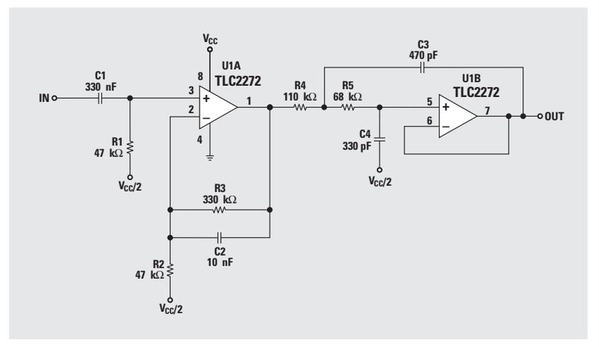
This circuit topology is very flexible. Most of the RIAA breakpoints are independently adjustable, as follows:
