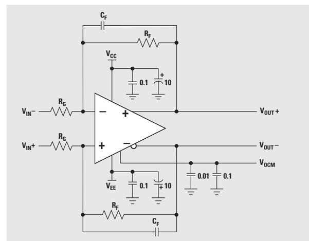
Figure 10. First-order active low-pass filter with passive second pole
