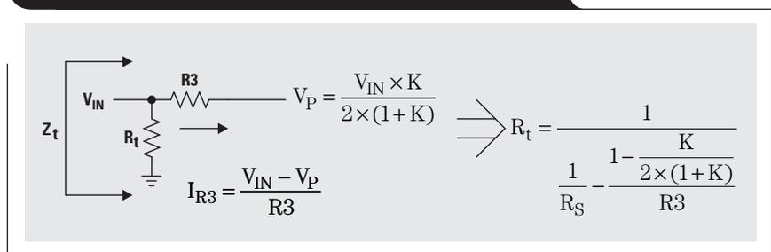
$$\frac{V_{IN}}{I_{R3}} = \frac{R_3}{1 - \frac{K}{2 \times (1 + K)}}$$
