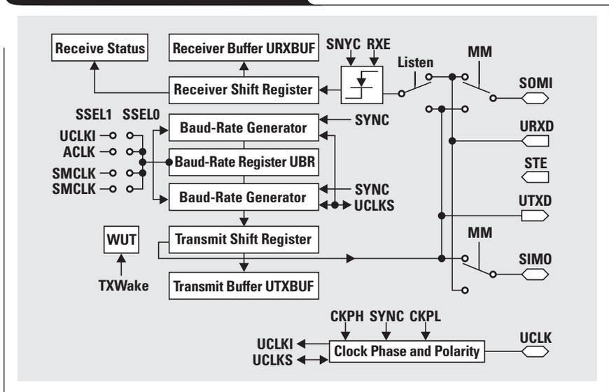
**Figure 3. MSP430F149 special-function registers used with USART0**
