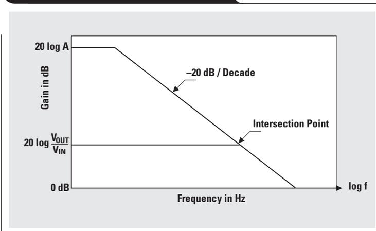
guaranteed minimum specification is 90 dB; hence the typical curve is reduced by  $116 \text{ dB} - 90 \text{ dB} = 26 \text{ dB}$  to turn Figure 4 into a guaranteed curve—i.e.,  $107 - 26 = 81 \text{ dB}$  at  $f = 10 \text{ Hz}$ . The data for the new curve is given in Table 1.
