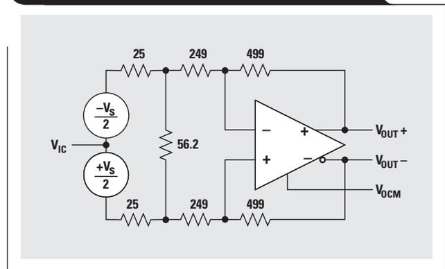
Figure 5. Terminating a single-ended input signal
