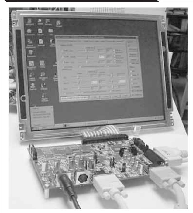
The data of the top ADC also feeds the THS8134 DAC. Note that 48 signal lines are provided from each ADC, since each ADC has three double-pixel-width buses (3 channels x 8 bits x 2). The DAC has only 3 x 8 input signals. For the DAC to work, the 24-bit output needs to be selected.
