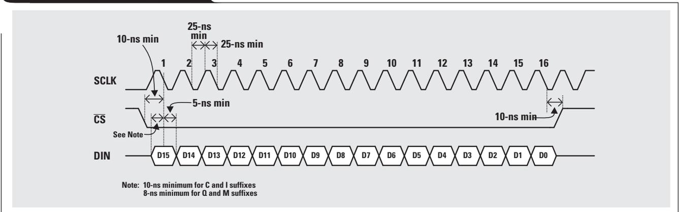
**Figure 6. ADC and DAC timing diagram**
