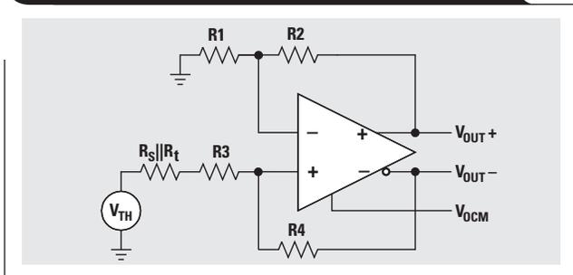
As an example, suppose you are terminating a 50- $\Omega$  single-ended source and want an overall gain of 1 from the source to the differential output of the amplifier. Start the design by first choosing the value for  $R_3$ , then calculate  $R_t$  and the feedback resistors. This will be an iterative process, starting with some initial assumptions that are then refined.
