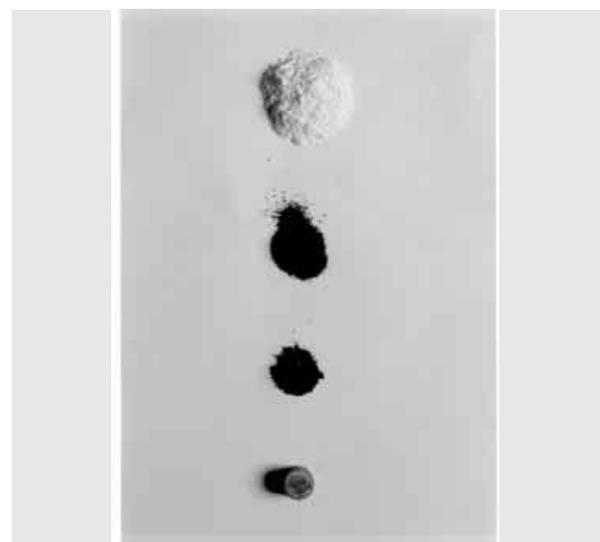
The light-colored powder at the top is raw precursor. Below that is pre-sintered powder before and after it is finely ground and filtered. The weight loss that results is evident. Compressing the sintered precursor in a hydraulic press produces the finished thermistor.
