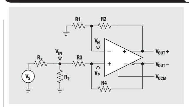
Figure 6. Single-ended termination ac impedance
