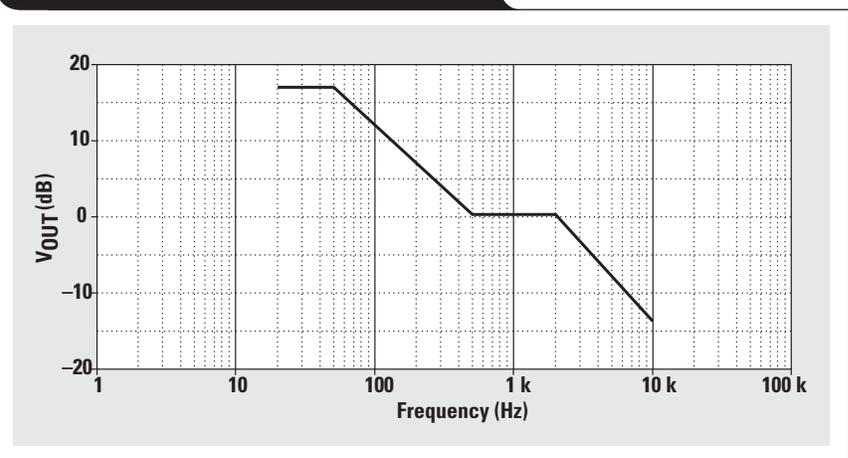
Figure 10. RIAA equalization circuit
