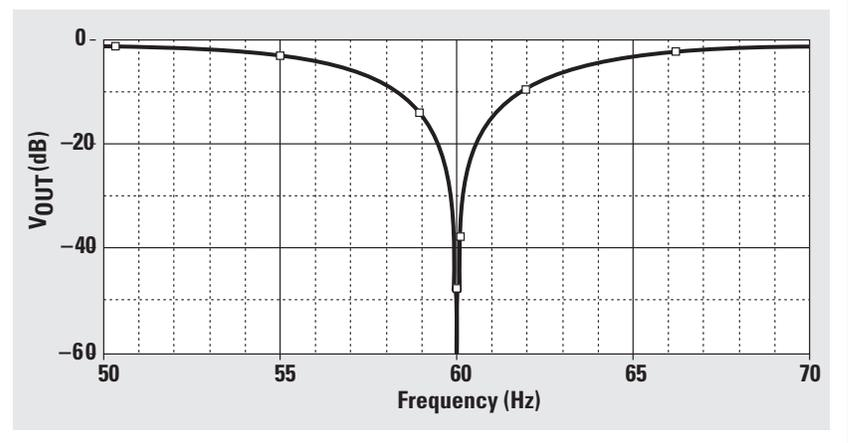
Figure 3. Varying notch depth
