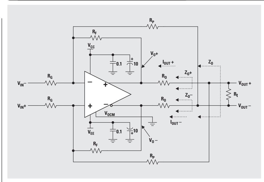
$R_0$  and  $R_t \parallel 2R_P$ , the gain from  $V_{IN} = (V_{IN+}) - (V_{IN-})$  to  $V_{OUT} = (V_{OUT+}) - (V_{OUT-})$  is
