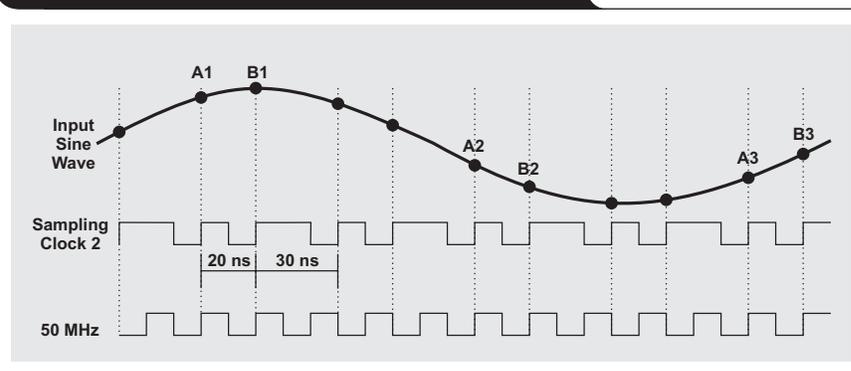
**Figure 5. ADS826 non-uniform sampling performance analysis for Case 2**
