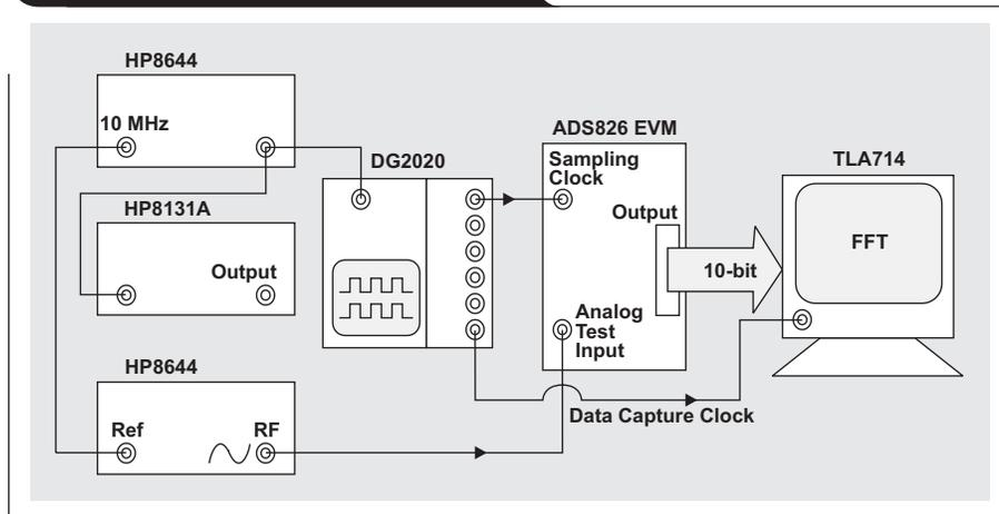
Figure 2. Pattern clocks for ADS826 test
