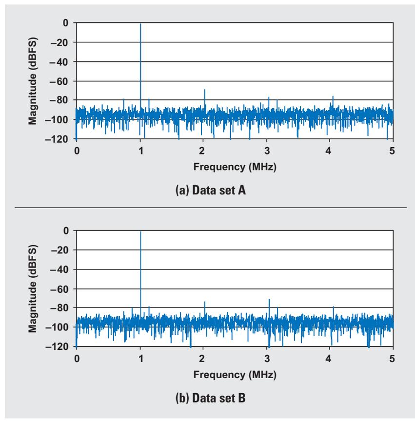
**Figure 10. Case 3 FFT outputs with 7.14-MHz downsampling frequency**
