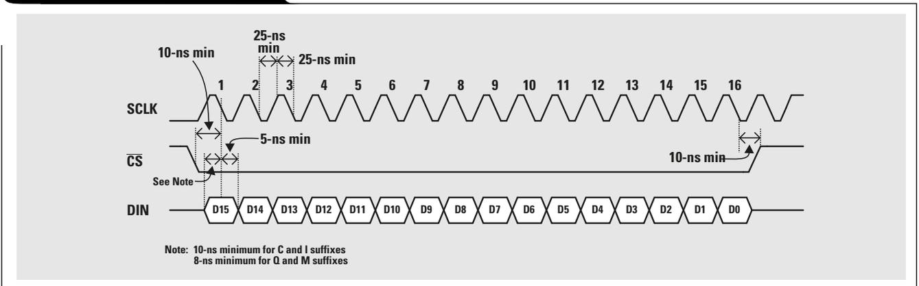
**Figure 6. ADC and DAC timing diagram**
