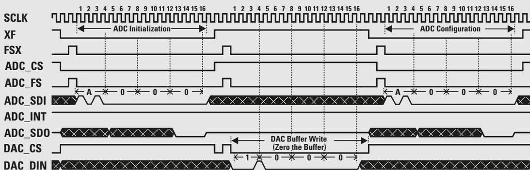
**Figure 9. ADC channel select, first conversion cycle, and DAC write**
