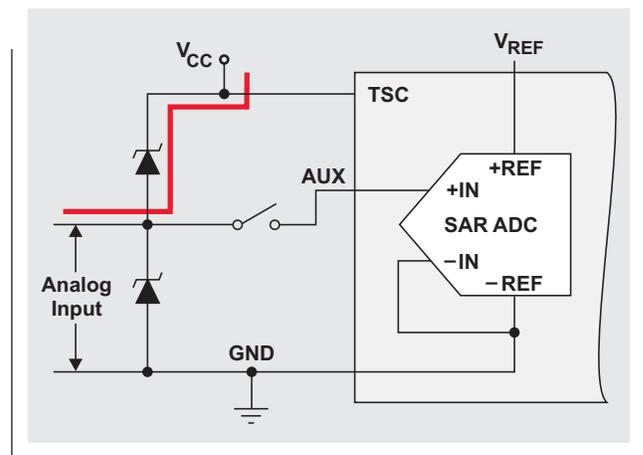
the analog input signal is active (AUX is nonzero) when the TSC is powered down ( $V_{CC} = 0$ ), the analog signal may be routed to the  $V_{CC}$  through the ESD-protection diode (see the red line in Figure 6). This may partially or fully power up the TSC, depending upon the amplitude of the input signal, consuming more power and possibly causing the TSC to malfunction. Thus the circuit configuration in Figure 6 should be avoided.
