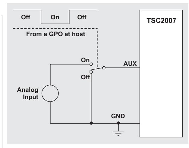
Some of TI's new TSCs, including the TSC2004/5/6/7, were designed with the enhanced, on-chip ESD protection shown by the simplified circuit in Figure 8. Obviously, for these devices, the input signal to the TSC's AUX should be removed before the TSC's  $V_{CC}$  power is shut down. An example of removing the AUX signal is shown in Figure 9.
