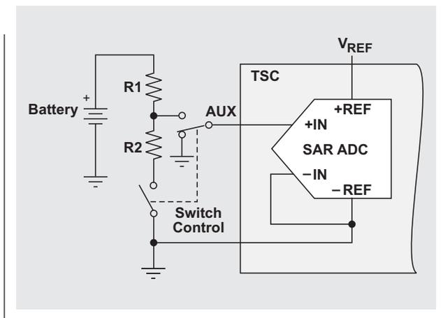
Similarly, while a TSC's AUX pin is used to monitor battery voltage, adding a controllable switcher like that shown in Figure 5 can reduce power consumption and ensure disconnection of the signal from the AUX pin while the TSC is powered down.
