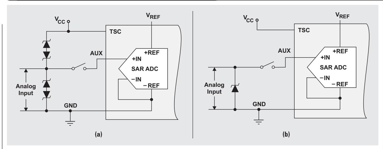
**Figure 8. TSC2004/5/6/7 internal ESD protection for AUX input**
