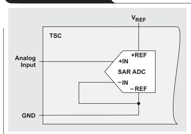
A TSC in differential mode does not need any reference, since the signal's driver is connected to +REF and -REF directly. However, the reference voltage,  $V_{REF}$ , is a must for SE operation and thus is always needed when an auxiliary input, such as the AUX or  $V_{BAT}$ , is measured.
