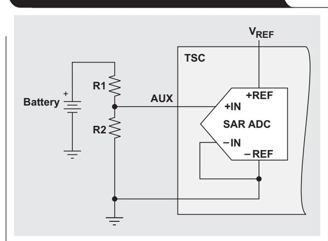
since the battery's voltage is normally higher than that of the TSC's power supply (and thus that of the  $V_{REF}$ ).
