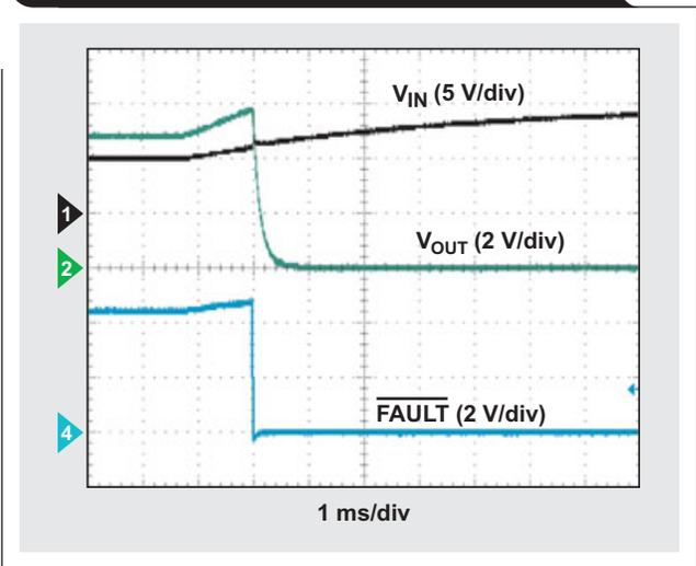
**Figure 5. Protective response of bq24314 to input overcurrent**
