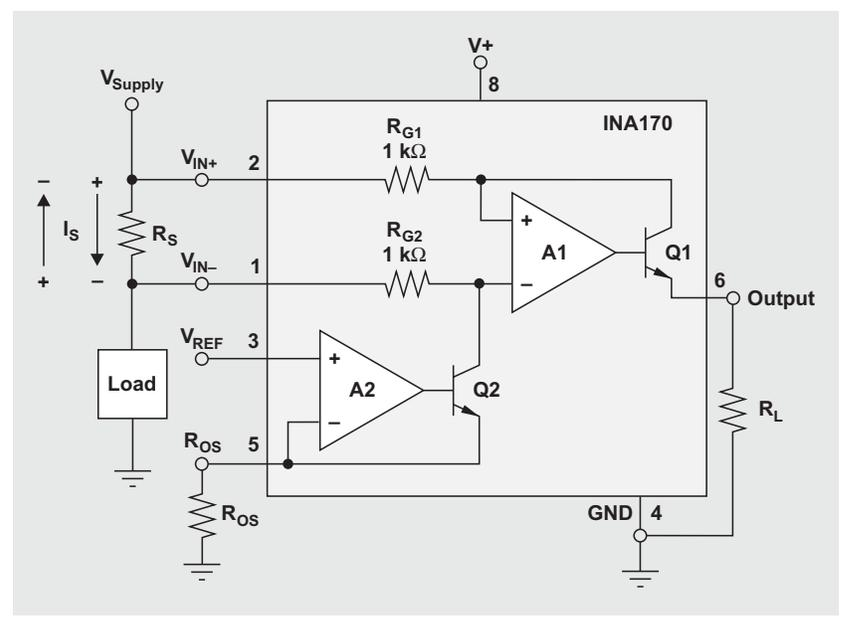
at the same CMV potential; but when a current flows through the shunt resistor, a differential voltage is developed and the inputs become separated by that amount. This voltage difference is amplified by the gain factor of the current-shunt monitor.
