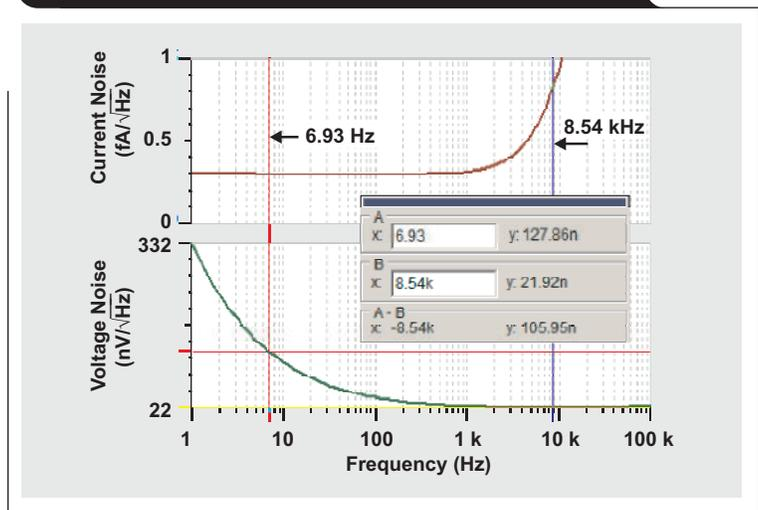
**Figure 12. TINA-TI model of Figure 6 circuit with noise sources added**
