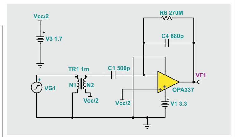
**Figure 7. Simulation of output noise from model in Figure 6**
