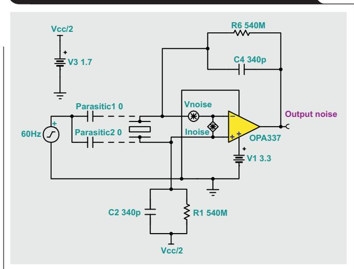
**Figure 18. Differential amplifier nearly eliminates common-mode noise**
