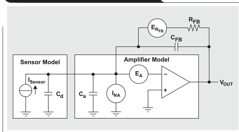
**Figure 5. OPA337's input-voltage and input-current noise**
