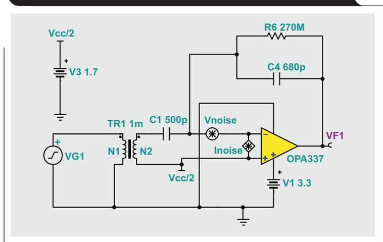
**Figure 13. Simulation of output noise from circuit in Figure 12**
