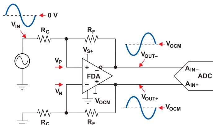
**Figure 1. Single-Ended Bipolar Input Circuit**
