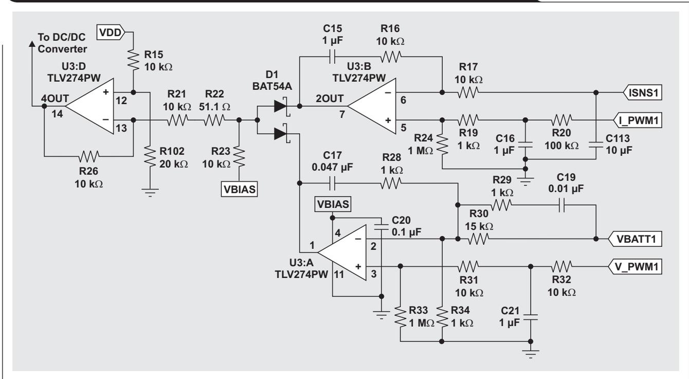
Figure 3. Overvoltage and reverse-polarity protection circuitry
