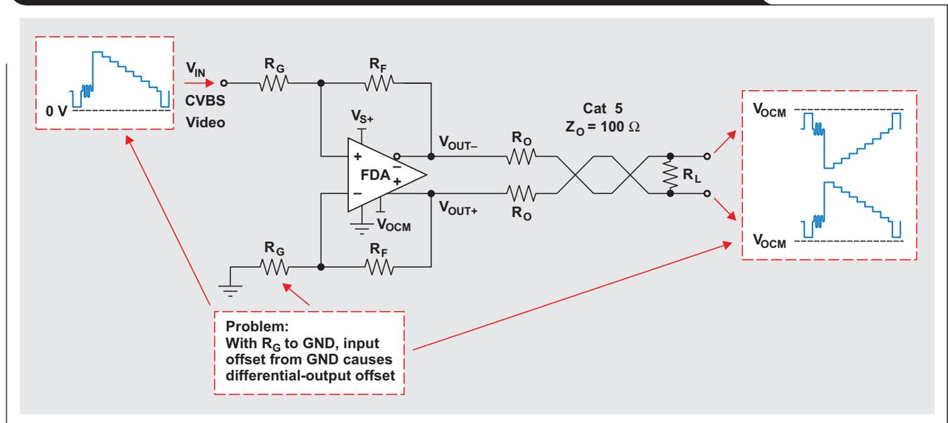
**Figure 3. Proposed circuit #2 with corrected differential-output offset**
