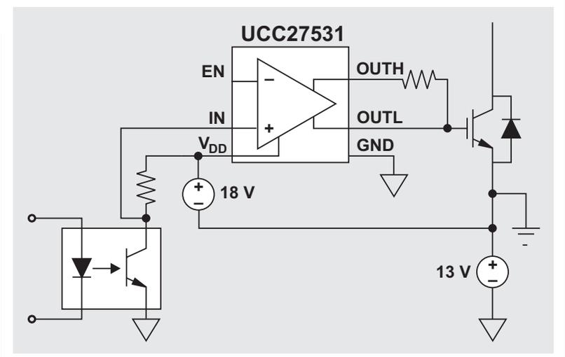
Since the UCC27531 is a rail-to-rail driver, OUTH pulls up the power-switch gate to its  $V_{DD}$  of 18 V relative to the emitter. OUTL pulls down the gate to the driver's GND of -13 V relative to the emitter. The driver effectively sees +18 to -13 V, or 31 V from  $V_{DD}$  relative to its own GND. Further, the 35-V rating provides a margin to prevent overvoltage failure of the IC due to noise and ringing.
