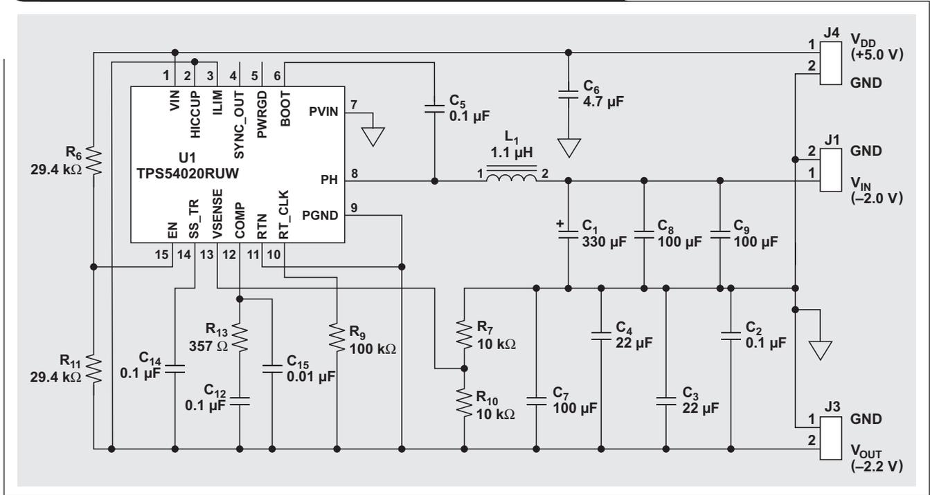
The significance of these similarities is that the negative boost converter can be constructed by using a readily available positive buck converter. One difference in operation is that the boost converter has a discontinuous output current and a continuous input current, the opposite of the buck converter.
