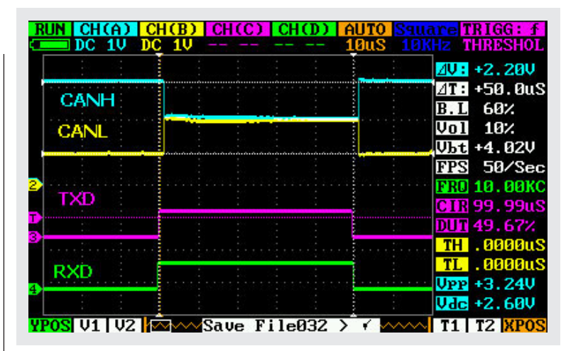
Figure 7. TI CAN EVM signals
