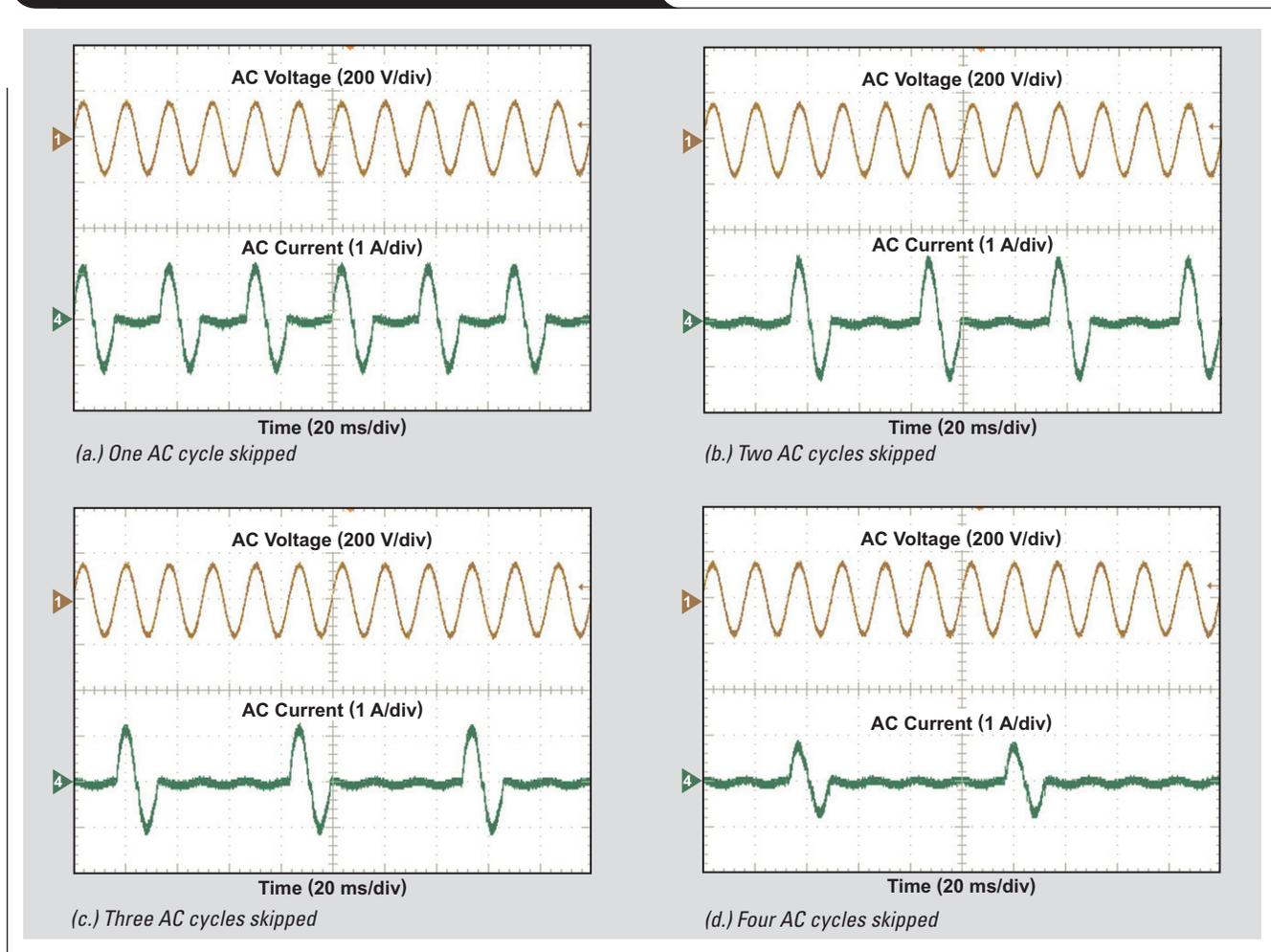
the PFC now operates at middle load or completely shuts off to skip AC cycles, the light-load efficiency is increased and THD is reduced. Figures 4 and 5 show the efficiency and THD improvements with this special burst-mode.
