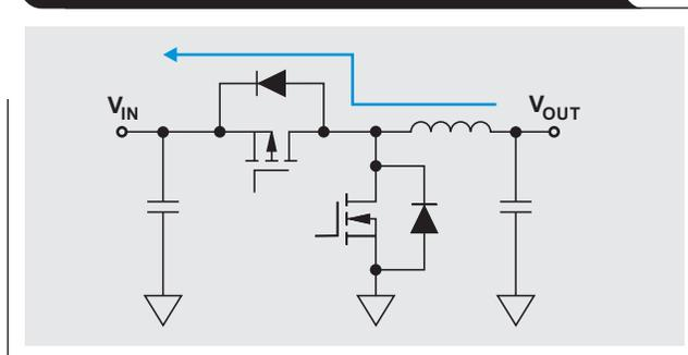
**Figure 3. The input diode blocks the input supply rail from voltage applied to the output**
