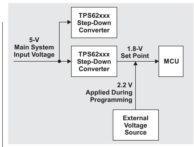
If the main supply voltage is the AC line voltage, for example, it may be physically unsafe for an operator to apply this voltage to the system during production when all safety mechanisms are not yet installed. Also, if the system contains motors or heating elements, powering up the full system may activate these sub-systems in unsafe ways. Applying an external voltage is still a common method for programming the MCU.
