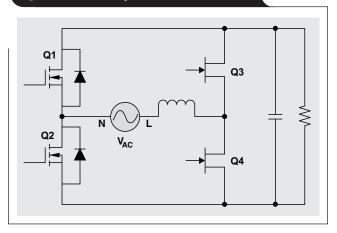
peripherals, is a good candidate for this topology. Even though the traditional control method cannot be directly applied to a totem-pole PFC, special control algorithms need to be developed. In fact, the control of a totem-pole PFC is much more complex when compared to a traditional PFC. Lacking a bridge rectifier, the bidirectional inductor current and the function swap between the main switch and the sync switch creates many challenges in a totem-pole PFC design.
