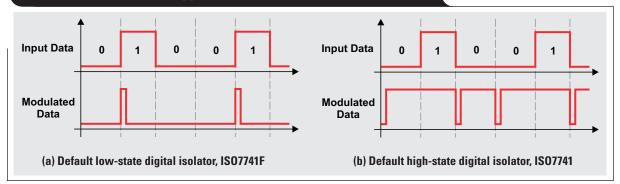
require the bus to be in a particular state (either high, low or custom) during this idle state.
