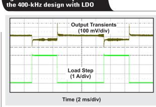
A faster switching frequency and faster loop bandwidth enabled a much faster transient-response time and reduced voltage undershoots and overshoots. Table 5 shows the results.
