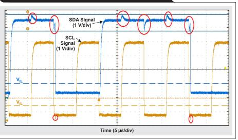
lines as low. Figure 3b shows  $V_{OL}$  higher than  $V_{IL}$  but also lower than  $V_{IH}$ . The SDA/SCL line in Figure 3b is in an unknown state, which is not allowed in  $I^2C$ . The signal may be interpreted by the receiving device as a low or high, depending on the design of the device's input stage.
