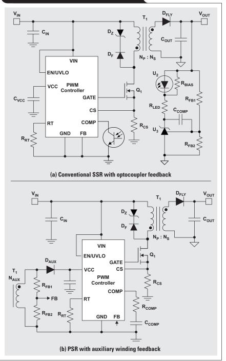
amplifier (often implemented as a TL431 shunt-regulator device), associated resistors and capacitors for the feedback divider and compensation, and the optocoupler for secondary-to-primary feedback. Only one component, the transformer, crosses the isolation barrier. PSR also removes the associated biasing losses of an optocoupler and the TL431.
