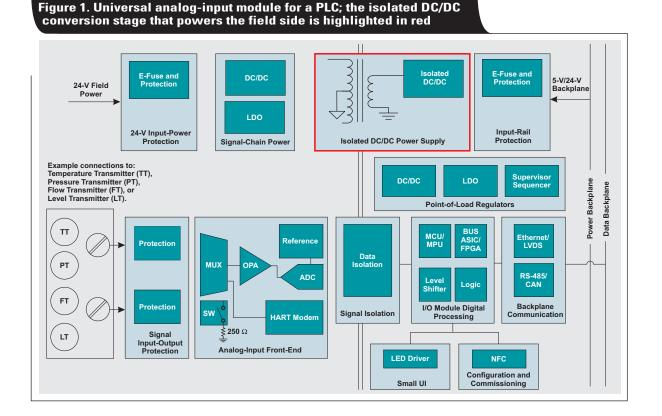
The analog front end shown in Figure 1 is galvanically isolated from the embeddedprocessing subsystem to break ground loops between the module and its sensor inputs or remotely connected systems. Signal isolation also improves measurement accuracy, as it removes noise and helps with electrostatic discharge, electrical fast-transient and surge protection of the inputs.<sup>[5]</sup>
