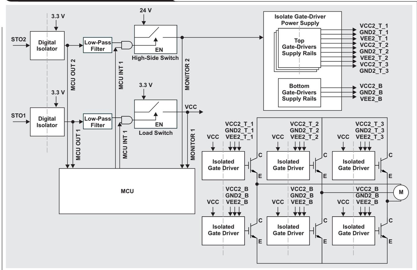
Table 4 highlights some of the diagnostic capabilities of the STO design when both STO signals are generated by external devices. The 1oo2d architecture helps achieve a HFT of 1. Only the occurrence of two simultaneous faults can cause failure of the safety function.
