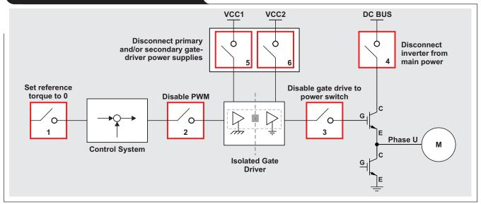
Figure 2 is a block diagram of the STO function for complementary metal-oxide semiconductor (CMOS) input-isolated gate drivers and logic-supply voltages, providing an HFT of 1. Implementing a hardware shutdown across channels by using a three-input AND gate and taking a third input from the other channel's low-pass filter output helps further enhances safety.
