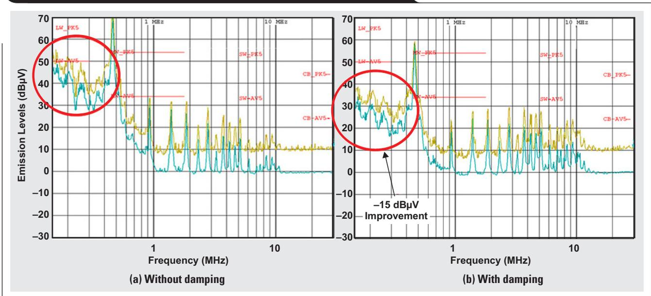
Figure 5 demonstrates a reduction in EMI when implementing a parallel RC network as outlined in Equations 3 and 4.
