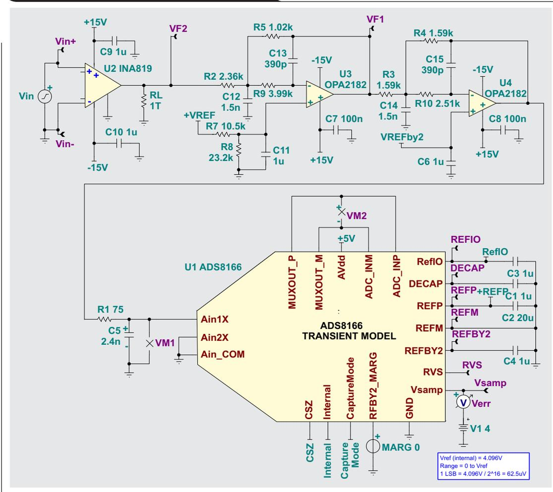
**Figure 6. TINA-TI software simulation results: INA819 and OPA182 filter DC sweep**
