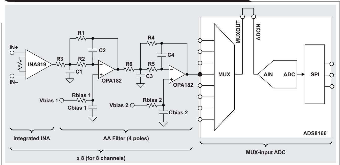
The external resistor sets the gain (G) for the INA819 or will not be populated for a G = 1. The system-level error budgeting is fairly complex for an instrumentation amplifier: Reference 4 provides a comprehensive analysis. The fourth-order filter is constructed using two stages of the multiple-feedback active filter type. Multiple feedback filters:
