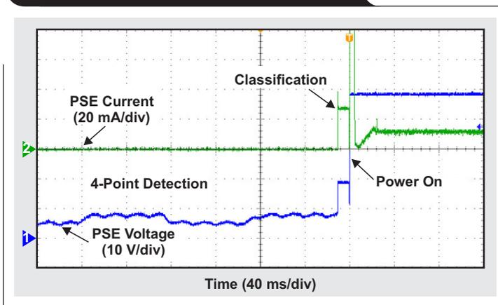
For IEEE 802.3at devices, this procedure is extended. A first classification with a current of 36 mA to 44 mA signals Class 4 IEEE 802.at devices and must be followed by a second classification. This power class allows up to 30 W.<sup>[5]</sup>
