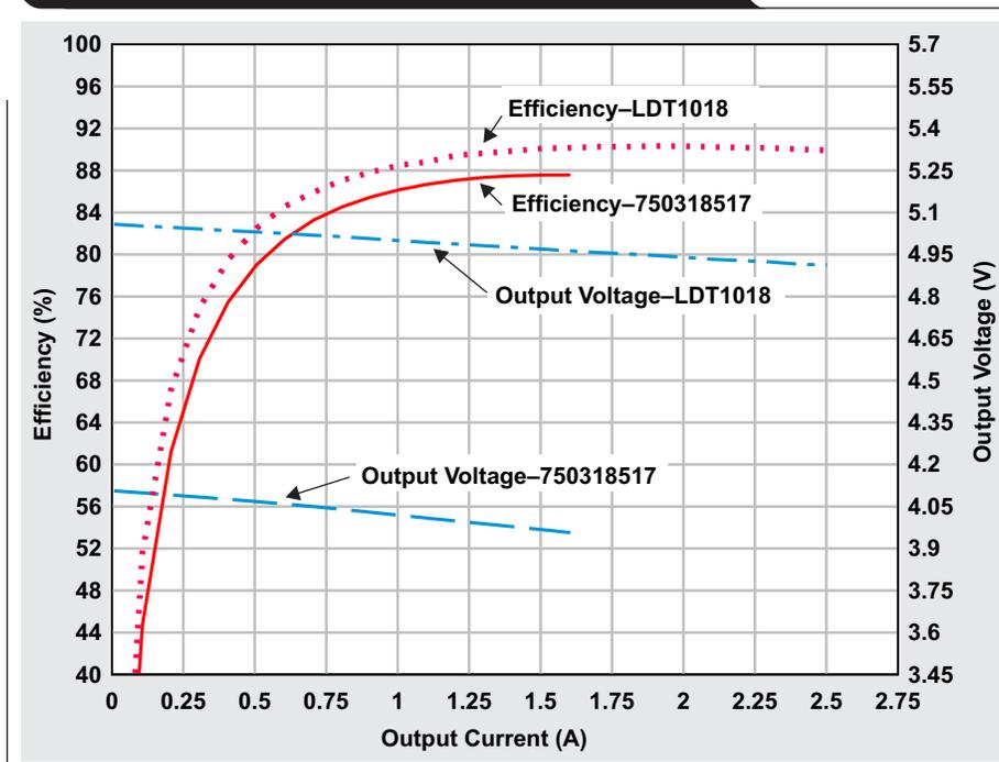
Power dissipation is critical in this type of application, making the replacement of the rectification diode on the secondary side a factor. Together with primary-side feedback, a diode rectification shows a current- and temperature-dependent voltage drop. In most applications this is not critical, but when the flyback is designed for 5 V and should directly supply a power-management IC (PMIC) with a 5.5-V maximum input voltage, voltage overshoot at low currents can cause trouble.
