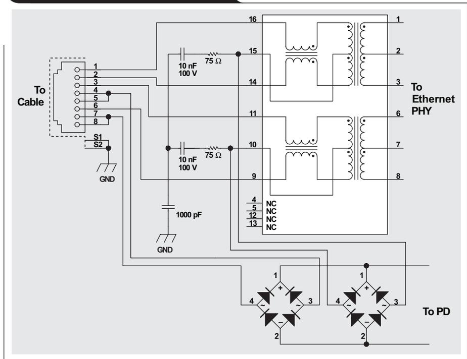
Figure 4. High-density reference design\* for isolated-PoE and GigE machine-vision cameras and sensors
