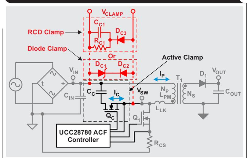
In addition to loss in the passive clamp, the QRF exhibits frequency-dependent losses at the switch node that are evident by examining Equation 2.
