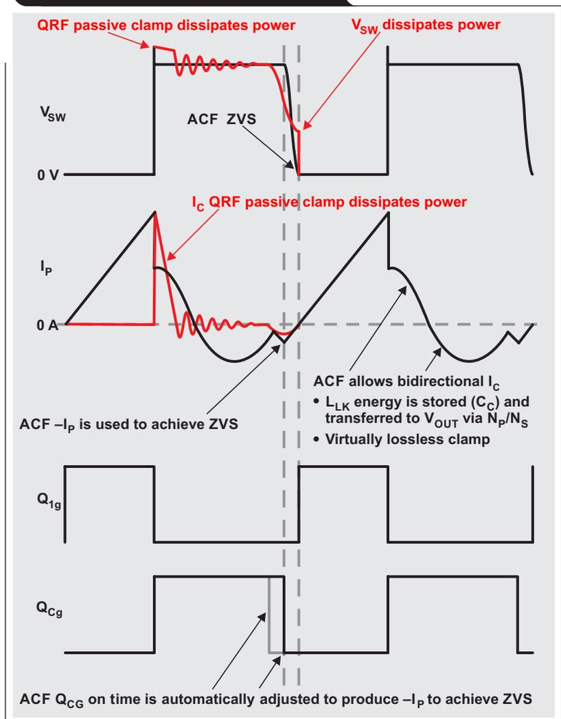
In addition, this approach can deliver efficiency greater than 94% and no-load power consumption of 60 mW. These figures are more than adequate to meet even the toughest CoC standards for standby power consumption.
