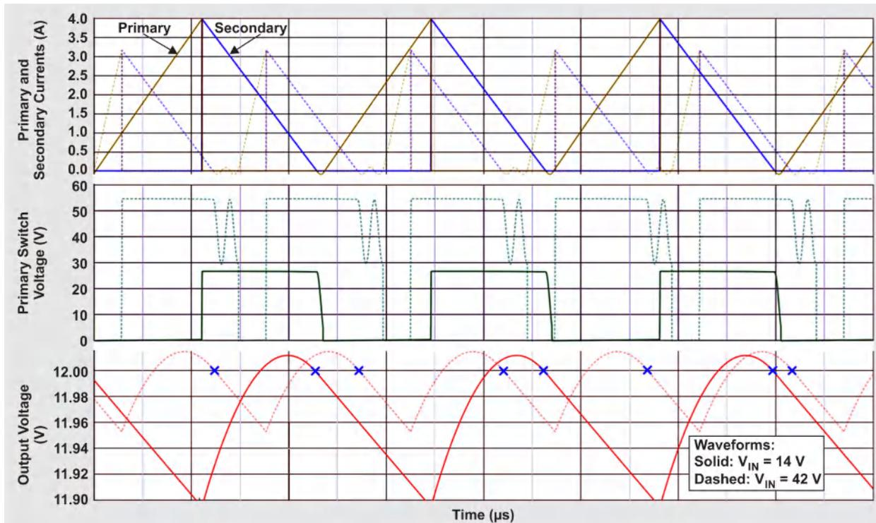
**Figure 5.** PSR Flyback Converter Waveforms at Input Voltages of 14 V (Solid Lines, BCM) and 42 V (Dashed Lines, DCM)
