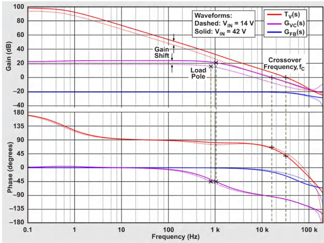
**Figure 6.** Simulated Bode Plots at Input Voltages of 14 v (Dashed Lines, BCM) and 42 v (Solid Lines, DCM)
