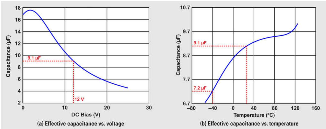
**Figure 4.** MLCC Plots for a 22-μF, 25-V, 1210, X7R Capacitor
