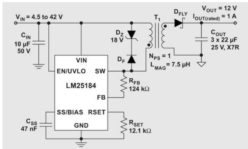
Figure 1. Typical Schematic of an Auxless PSR Flyback Converter
