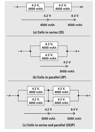
Figure 1. Voltage and Capacity Scaling for a Li-ion Battery
