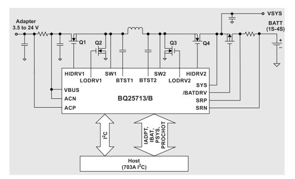
*Figure 3.* Charging Stage and Dynamic Power-path Management for a 4S Battery Pack
