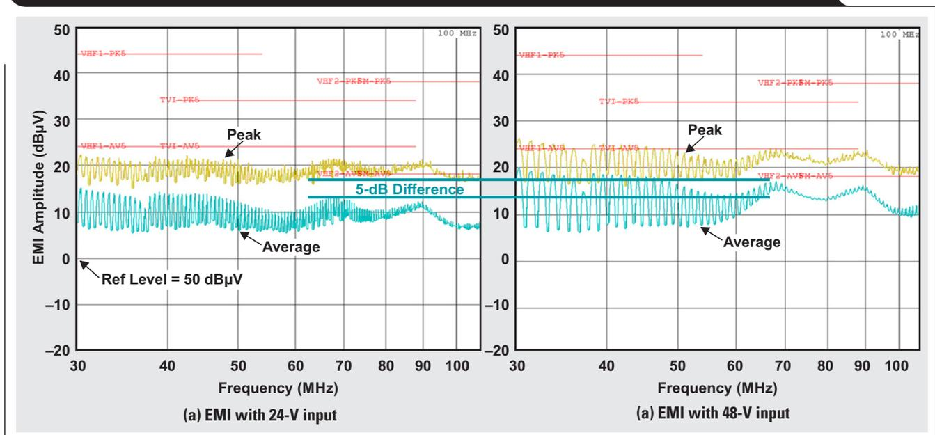
modulate at a more appropriate frequency for CISPR 25 Class 5, 30-MHz to 108-MHz testing. An effective modulation frequency can be achieved that's more broadband and better suited to a higher-frequency RBW filter (120 kHz) with PRSS.
