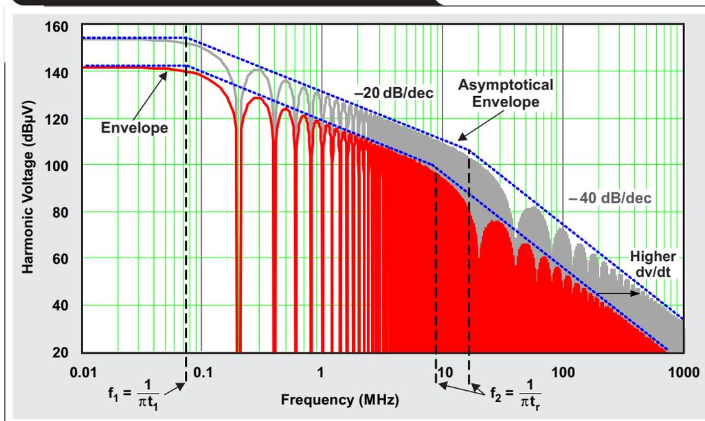
One method to reduce rise times involves creating a slower rise time of the MOSFET gate voltage by adding a series resistance with the boot capacitor ( $C_{BST}$  in Figure 4). The slower MOSFET turn-on will lead to a lower-frequency SW rise-time pole. Figure 5 demonstrates a 20-dB reduction using this method, with a switch-node voltage waveform having a rise time 100% larger than the default.
