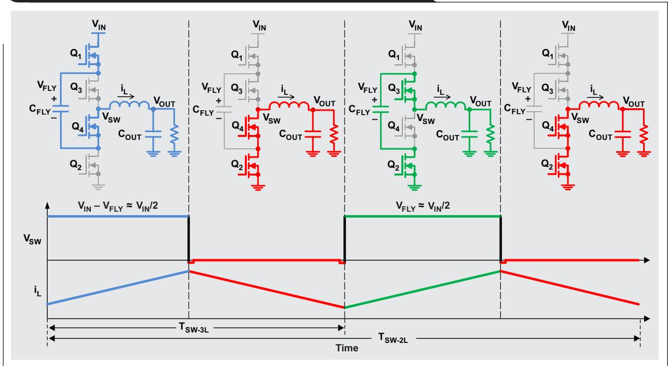
Figure 4. Three-level (3L) converter operation with D greater than 0.5
