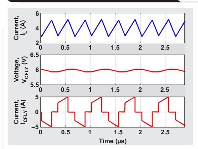
must withstand half the input voltage. Note that at  $D = 0.5$ ,  $I_{C(FLY)}$  sees the full load current.  $C_{FLY}$  capacitance is sized to keep  $\Delta V_{C(FLY)}$  less than 10% of  $V_{IN}/2$  in order to ensure loop stability. To ensure long capacitor life, the capacitor package size and RMS current rating must be large enough to handle the associated temperature rise.
