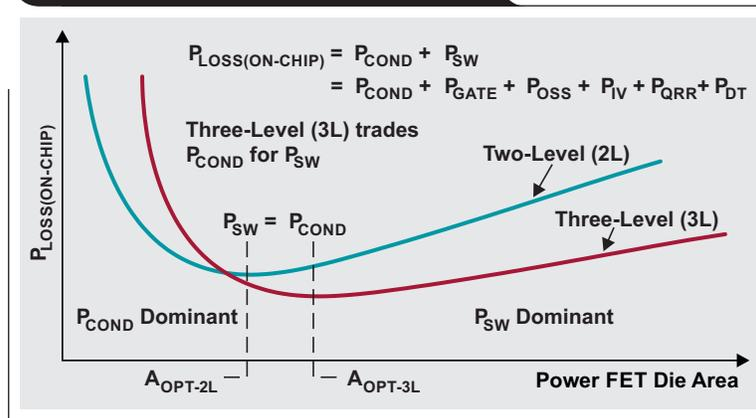
As shown in the far-right column of Table 1, for the same die area, the 3L topology conduction and dead-time losses double. But because the 3L FETs see one-half the input voltage compared to the 2L buck,  $P_{OSS}$  and  $P_{IV}$  losses are halved. An increase in FET area makes it possible to lower conduction losses until switching losses begin to dominate, as shown in Figure 5.
