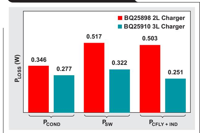
Figure 9a shows a plot of the BQ25910 and BQ25898 measured efficiency at a 9-V input voltage and a 3.8-V battery voltage. Figure 9b compares the losses of the two converters. At a 3-A charge current, the BQ25898 efficiency is 89.3%. From Figure 8, the BQ25910's  $P_{LOSS}$  is 0.850 W from a total output power of  $3\text{ A} \times 3.8\text{ V} = 11.4\text{ W}$ , resulting in 93.1% efficiency, which is very close to the measured 93.2%.
