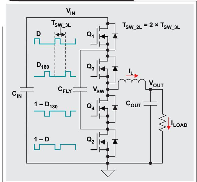
Figure 3. Three-level (3L) converter operation with D less than 0.5
