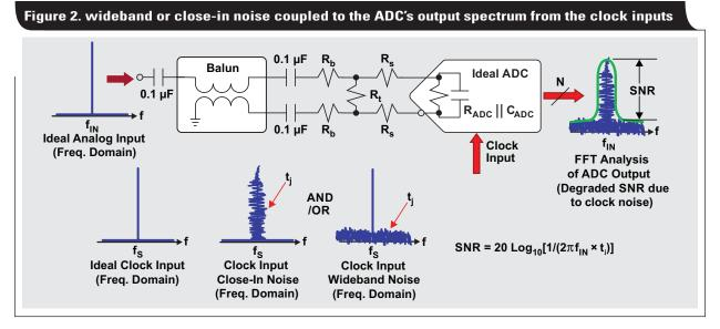
To illustrate this a bit more, if the clock has any wideband or close-in noise, then either noise can be a component evident in the output spectrum. This is illustrated in Figure 2. Earlier, it was suggested that the ADC be thought of as a giant mixer; even if the ADC is ideal, any noise that couples only to the clock in either a wideband or close-in fashion will ultimately convolve to the output spectrum.
