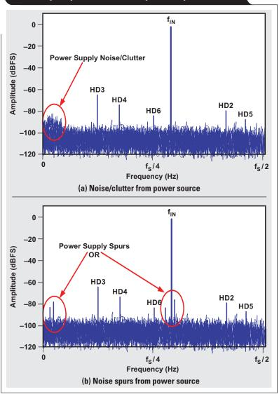
There is a slight difference in how noise couples through the clock versus how noise couples through the powersupply pins. In the clock example, the internal circuitry of the clocking nodes is well-tied into the sample-and-hold structures of the analog inputs. This makes it a perfect place for any noise or coupling through the clock pins to find their way into the internal signal path of the ADC as was shown in Figure 2. The coupling path is almost zero attenuation in this case.
