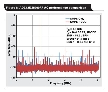
As shown in Figure 8, the ADC's AC performance (SNR/ SFDR) is on par between the two power supply designs as an analog input frequency of 1.5 GHz is applied while sampling at 10.4 GSPS. This basic test instills confidence that the SMPS design is robust and realizable.
